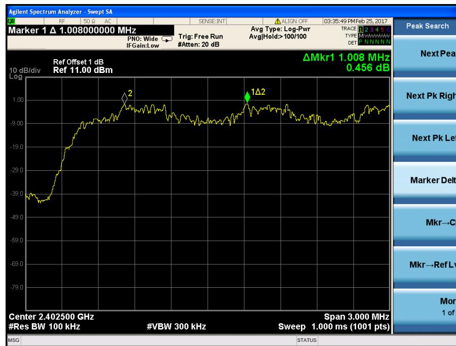
Channel Spacing (Middle CH=1MHz)
