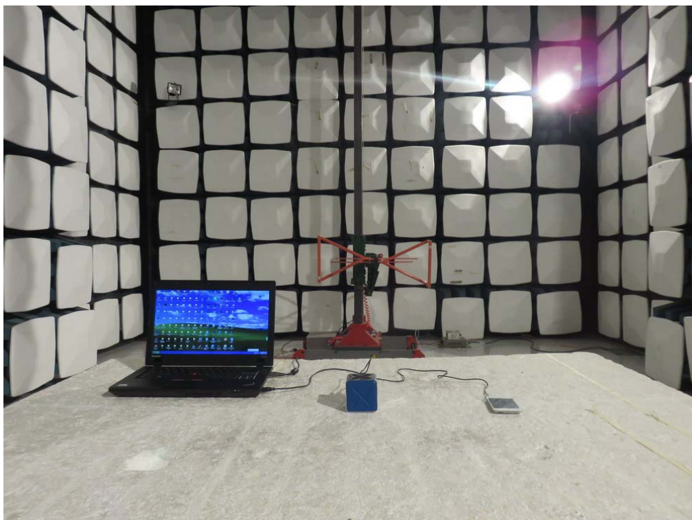
FCC RADIATED EMISSION TEST SETUP
