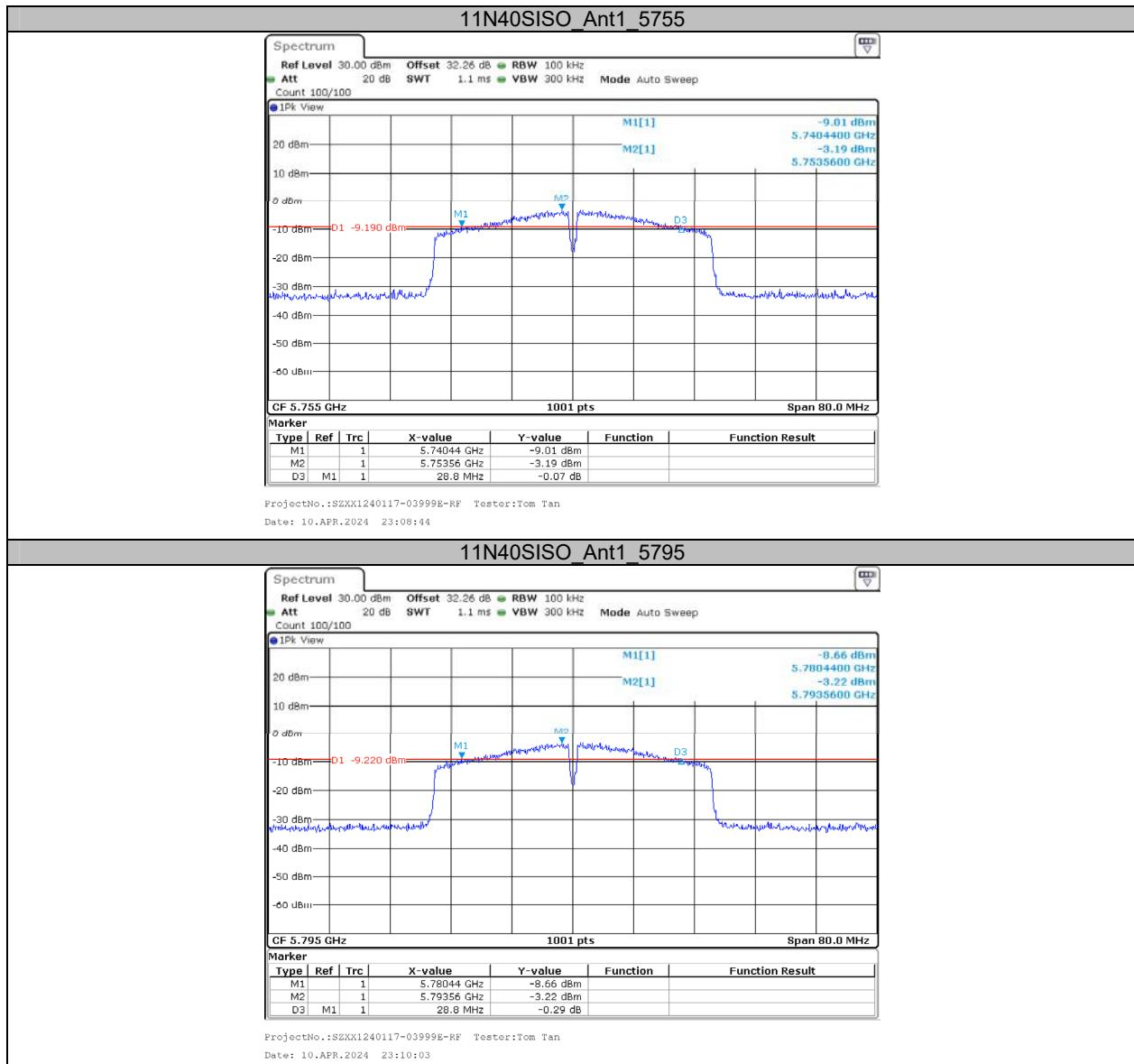
**Appendix D: Maximum conducted output power****Test Result**
