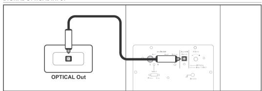
To use the «optical» input to connect our digital devices with help to optical cable. You can get a better audio quality with this input.
