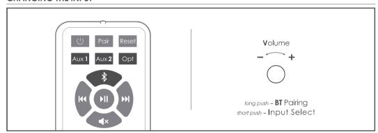
Inputs can be selected with the supplied remote control or with the «Volume Adjustment» on the back of the speaker.
