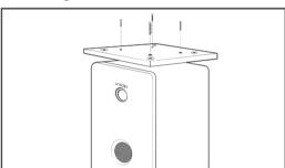
Carefully turn the cabinet over and place it on the packaging foams, or on a carpet, to avoid any damage of the top part. Take care not to damage the woodworking, the lacquered front or the drivers during this operation. Adjust the base on the cabinet and screw it using the four provided screws.
