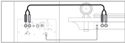
Connect your turntable to the RCA - AUX.1 input. Make sure that the phono or line input selector is in «PHONO» position.
