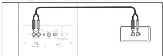
Connect any audio analog stereo source with RCA cable.
