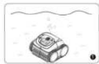
About 20 seconds of auto calibration on the floor, the indicator light will turn flashing blue. The cleaner is ready to clean.
