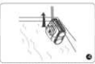
You can insert the included hook into a pool rod and lift the cleaner out of the pool.
