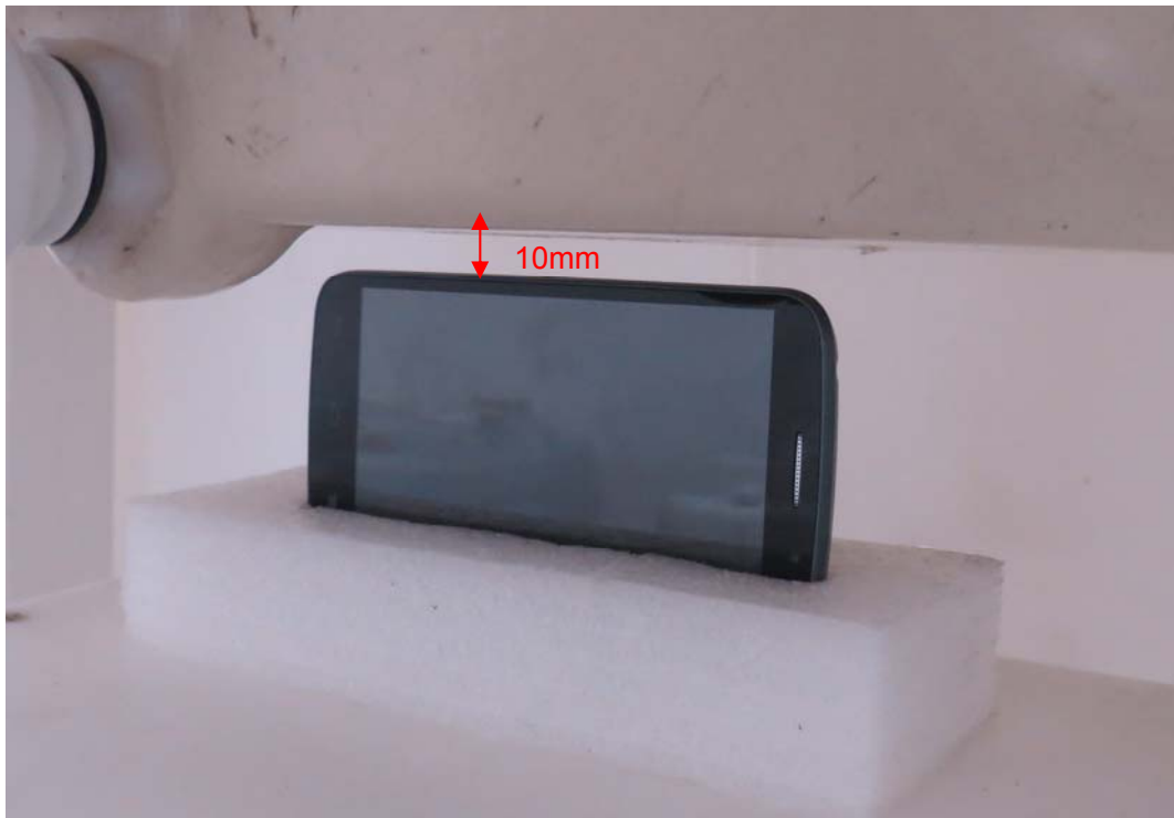
Picture 19: Left Edge, the distance from handset to the bottom of the Phantom is 10mm
