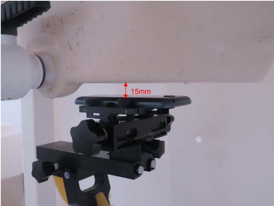
Picture 15: Back Side, the distance from handset to the bottom of the Phantom is 15mm
