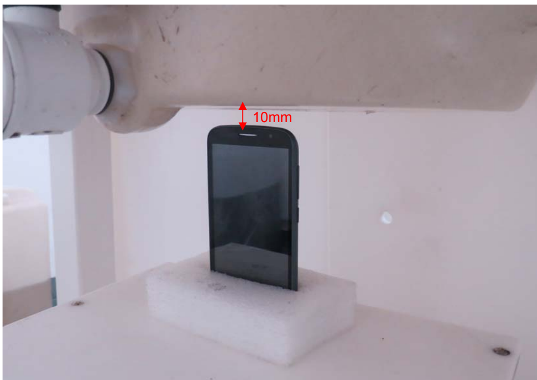
Picture 21: Top Edge, the distance from handset to the bottom of the Phantom is 10mm
