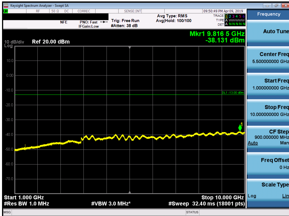
Plot 7-111. Conducted Spurious Plot (Band 12/17 - 10.0MHz QPSK - RB Size 1, RB Offset 0 - High Channel)
