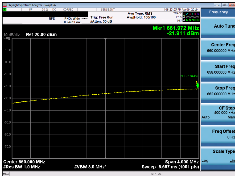
Plot 7-160. Lower Extended Band Edge Plot (Band 71 - 20.0MHz QPSK - Full RB Configuration)
