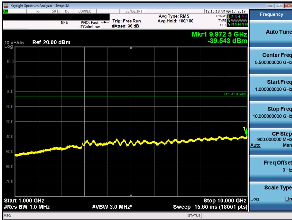
Plot 7-117. Conducted Spurious Plot (Band 26/5 - 10.0MHz QPSK - RB Size 1, RB Offset 0 - Low Channel)
