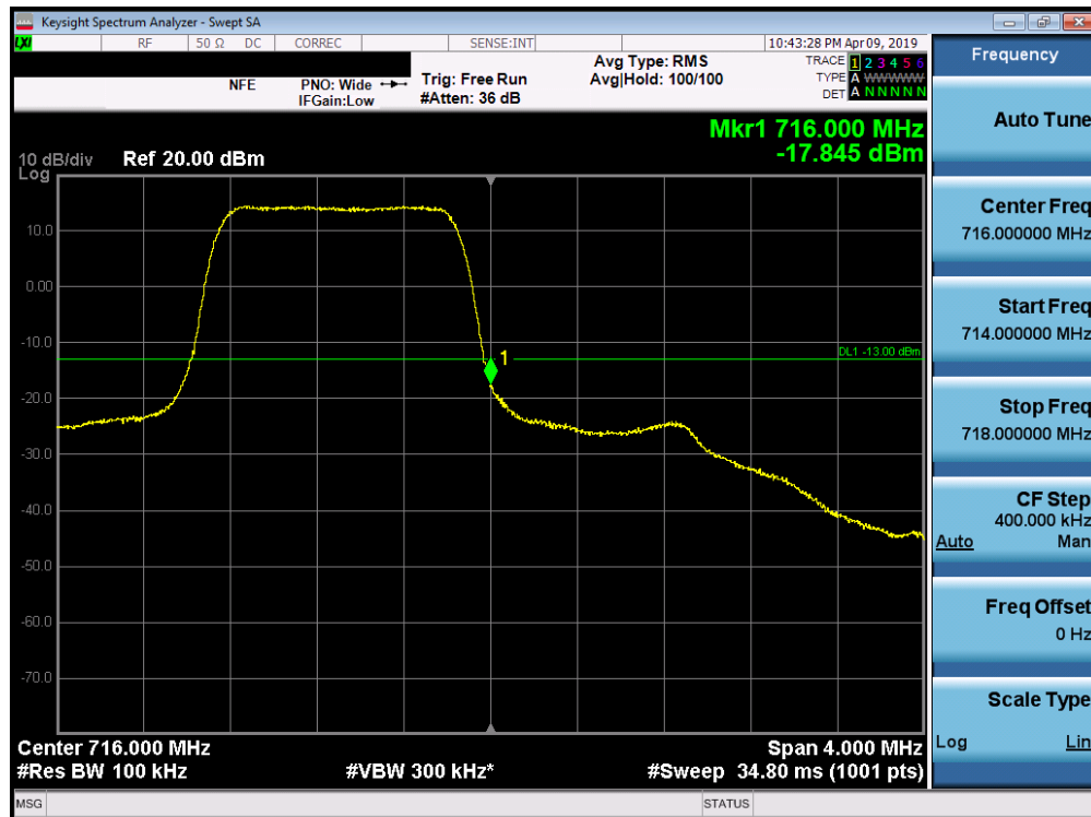
Plot 7-164. Upper Band Edge Plot (Band 12 - 1.4MHz QPSK - Full RB Configuration)
