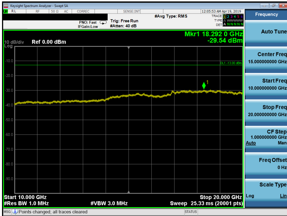
Plot 7-126. Conducted Spurious Plot (Band 66/4 - 20MHz QPSK - RB Size 1, RB Offset 0 - Low Channel)
