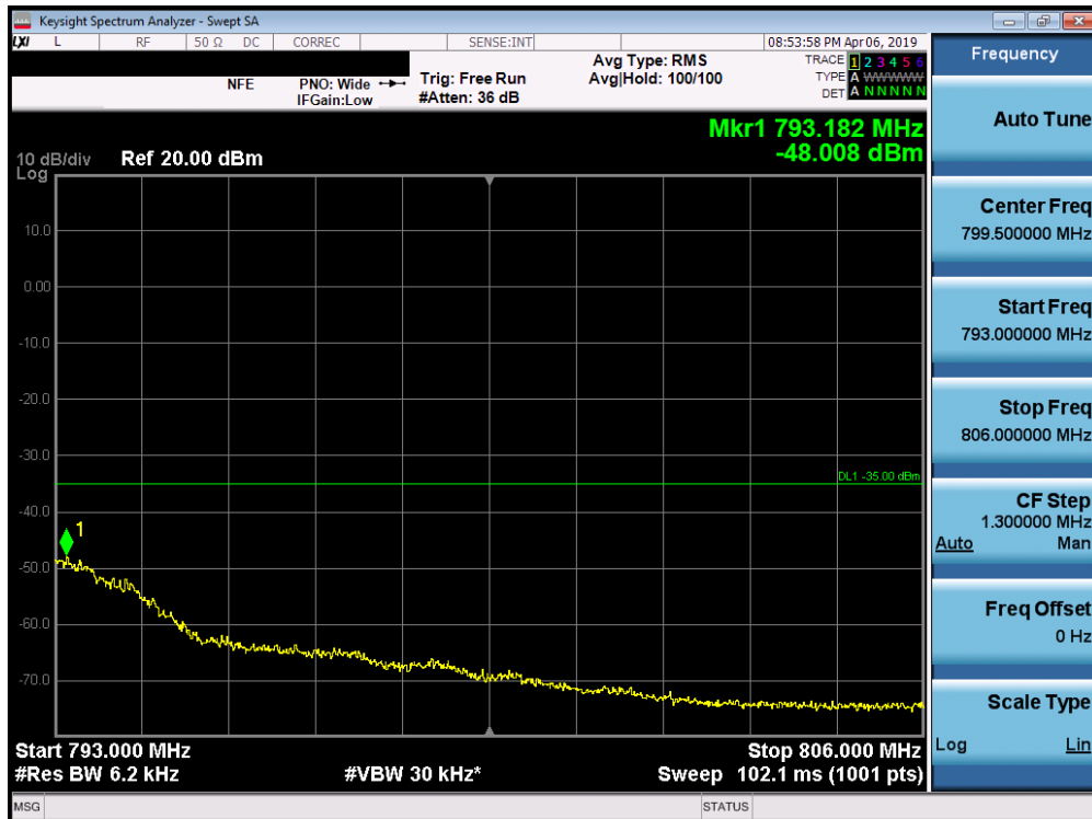
Plot 7-180. Upper Emission Mask Plot (Band 13 - 10.0MHz QPSK - Full RB Configuration)
