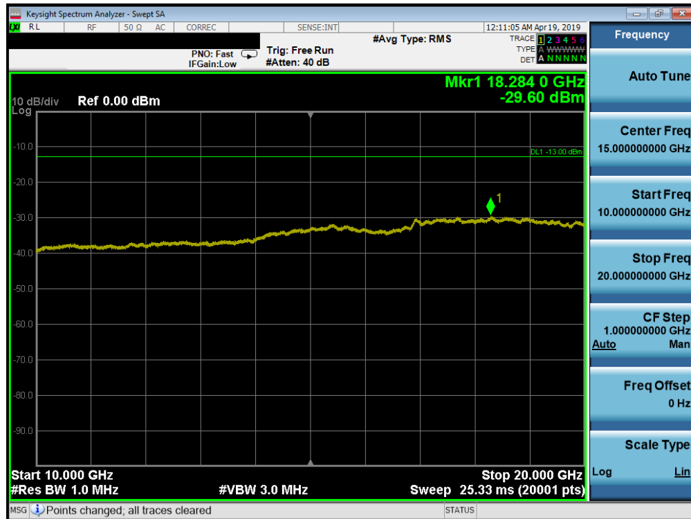
Plot 7-129. Conducted Spurious Plot (Band 66/4 - 20MHz QPSK - RB Size 1, RB Offset 0 - Mid Channel)
