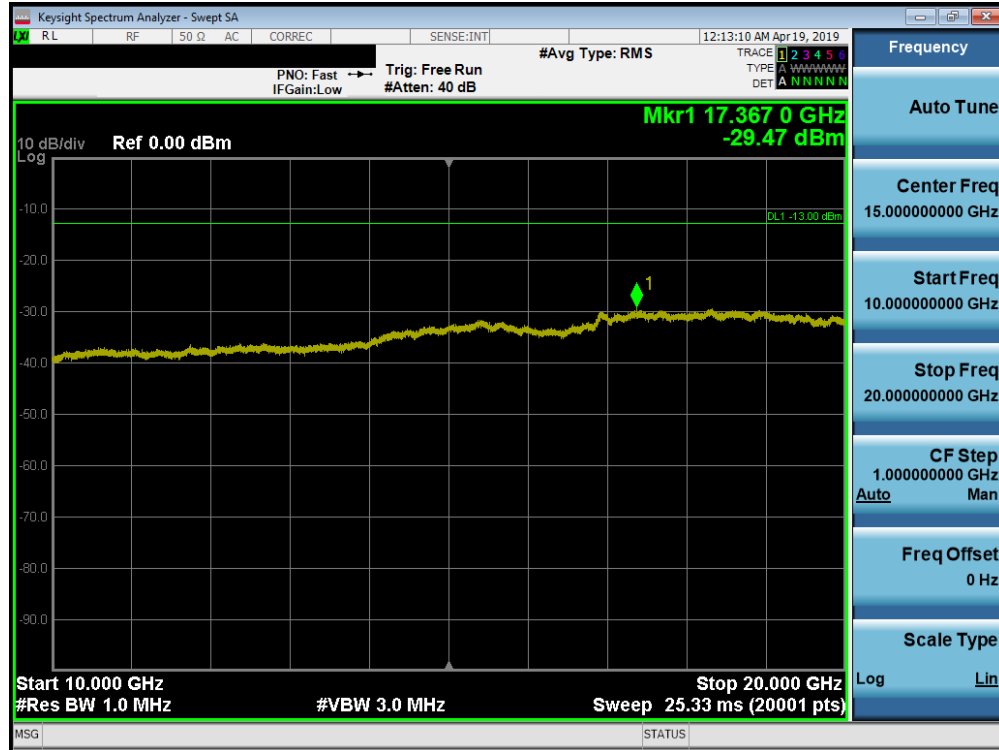
Plot 7-132. Conducted Spurious Plot (Band 66/4 - 20MHz QPSK - RB Size 1, RB Offset 0 - High Channel)
