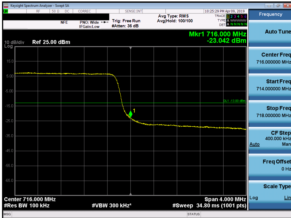
Plot 7-169. Upper Band Edge Plot (Band 12/17 - 5.0MHz QPSK - Full RB Configuration)
