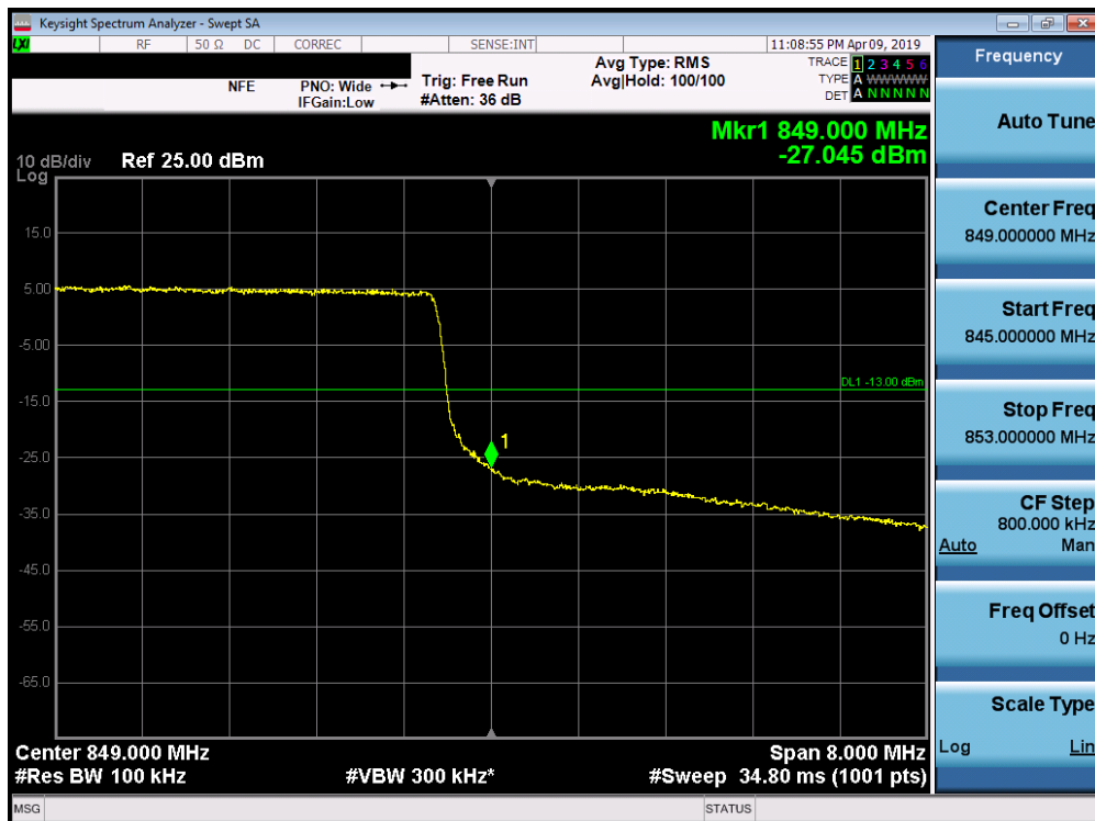
Plot 7-188. Upper Band Edge Plot (Band 26/5 - 10.0MHz QPSK - Full RB Configuration)
