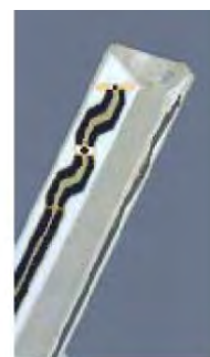
Figure E.2.2 Probe Thick-Film Technique
