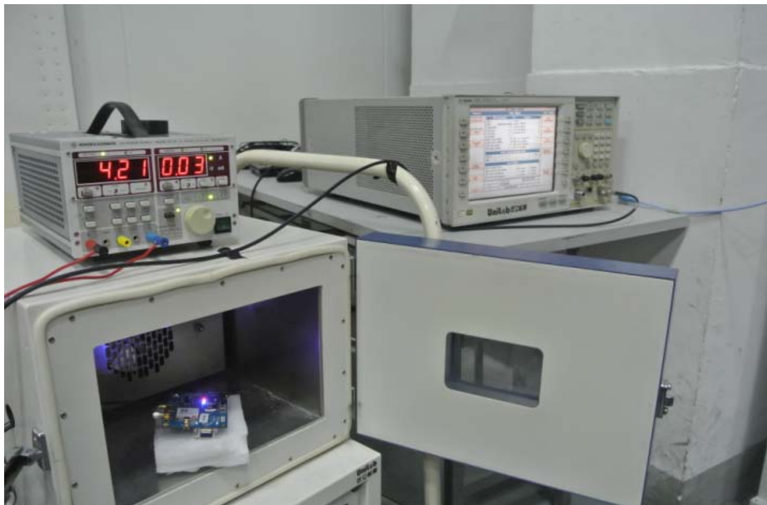
Frequency Stability Under Temperature & Voltage Variations Setup
