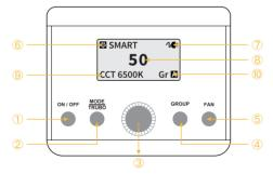
$\bigstar$  If there is no operation for 10 seconds, the current settings are automatically saved and the selection mode is exited.
