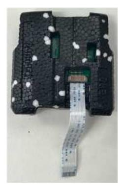
Connect the upper part with the BLEmodule to lower housing part with the interface board
