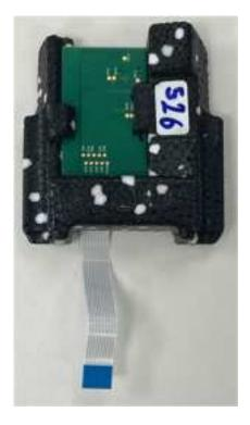
Mount the BLE-module holder in the upper part of the rotating laser housing
