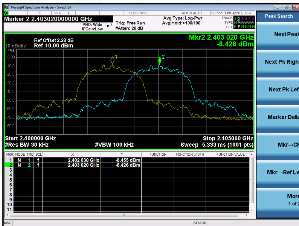
TEST PLOT FOR FREQUENCY SEPARATION
