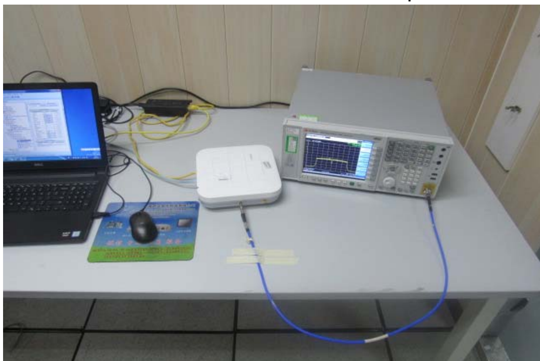
Picture 5 Conducted Test Setup
