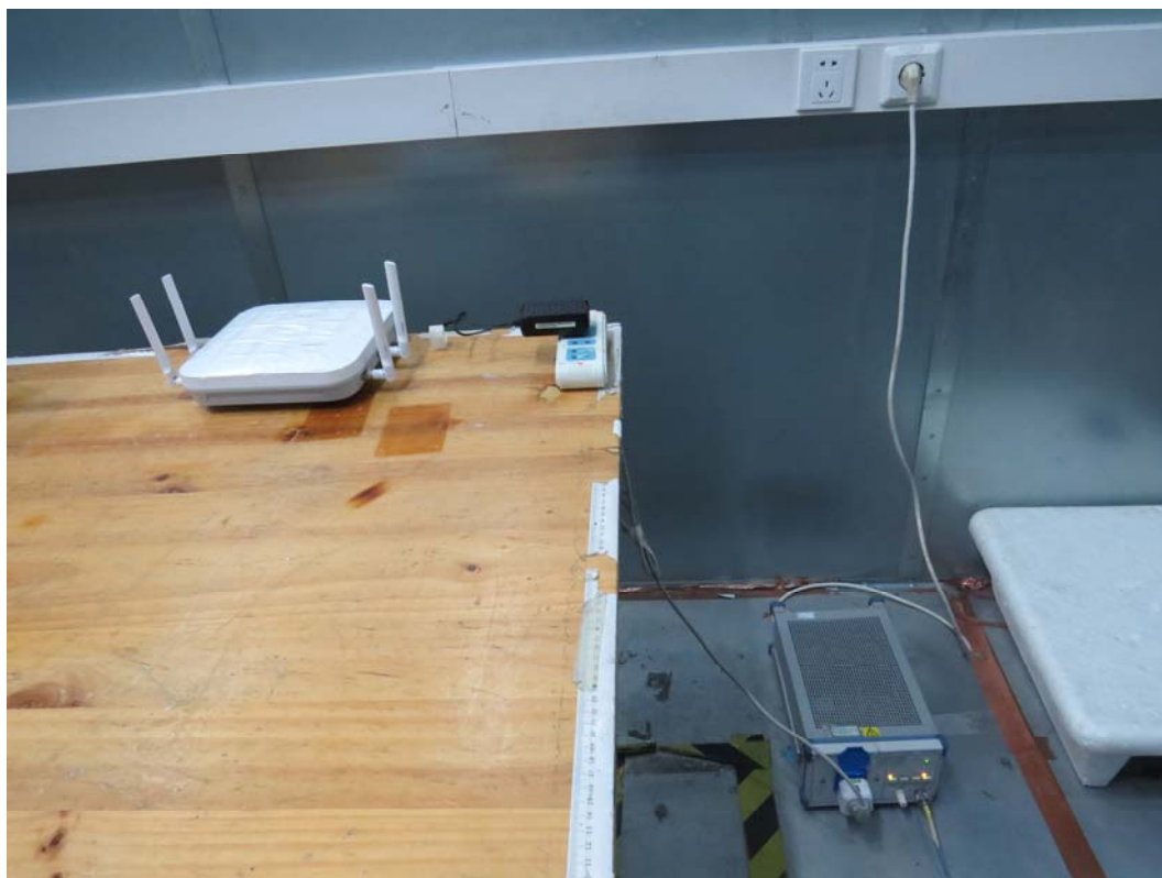
Picture 4 Conducted Emission Test Setup
