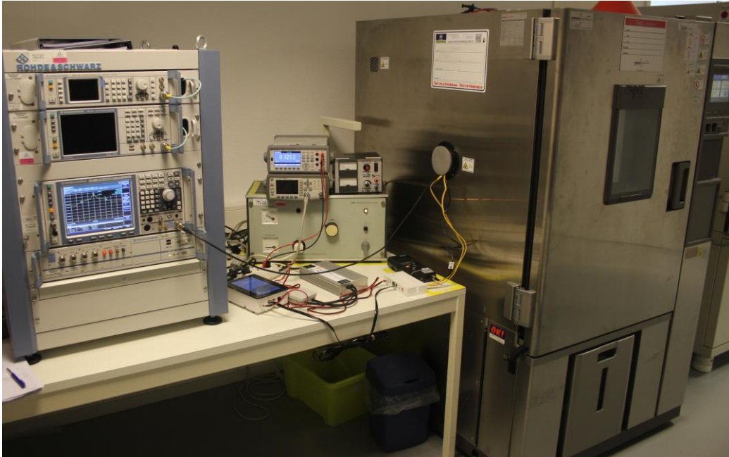
Photo 6 Photograph test setup Carrier stability
