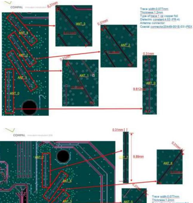
Trace width 0.077mm Thickness 1.2mm Type of bace 1 or copper fol Dielectric constant 4 53 (FR-4) Antenna connector Coasial connector20449-001E-03 I-PEX RITT
