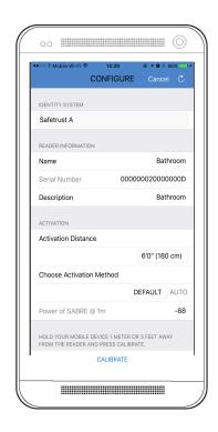
Select the Identity System, complete the location and description. Then calibrate the SLBRE. Once complete save the profile.
