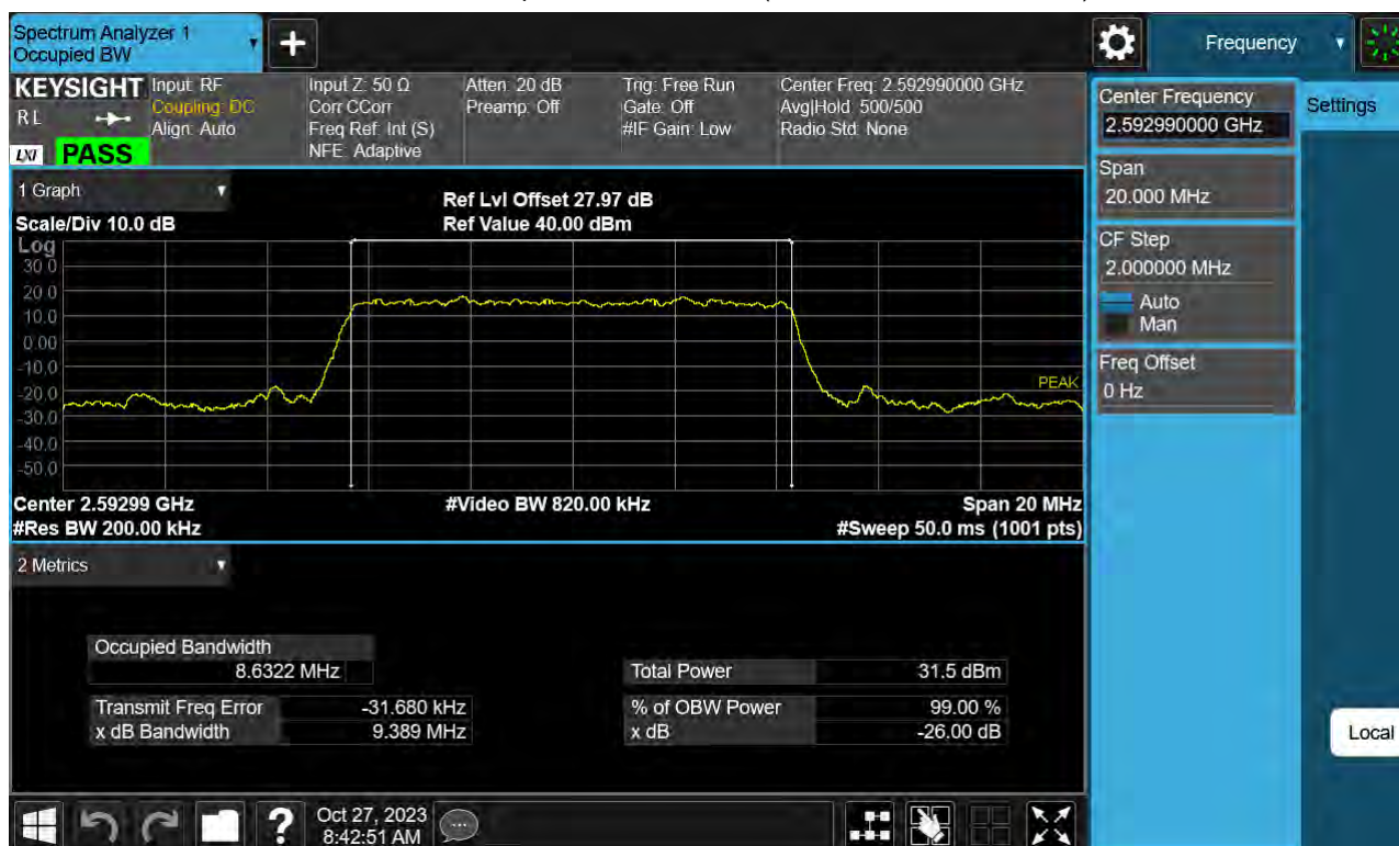
Sub6 n41. Occupied Bandwidth Plot (10 MHz Ch.518598 BPSK )
