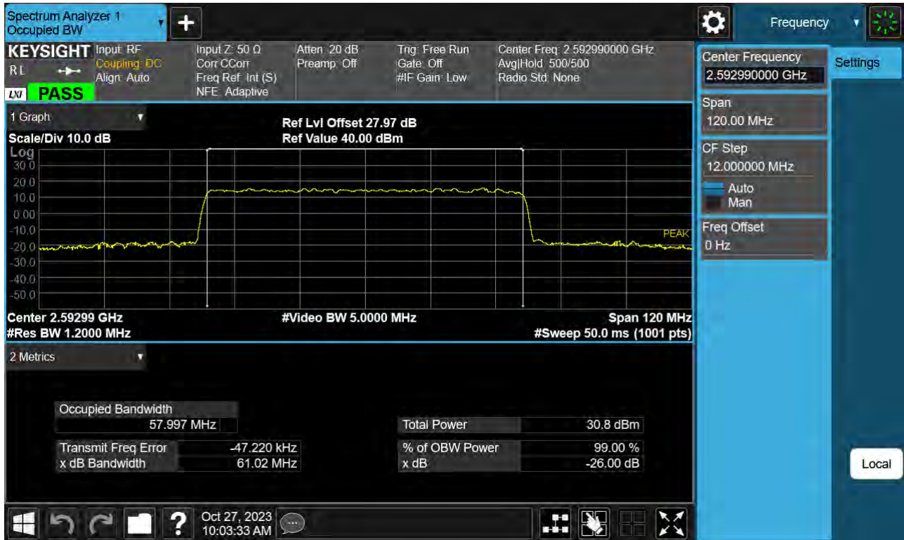
Sub6 n41. Occupied Bandwidth Plot (60 MHz Ch.518598 16-QAM )
