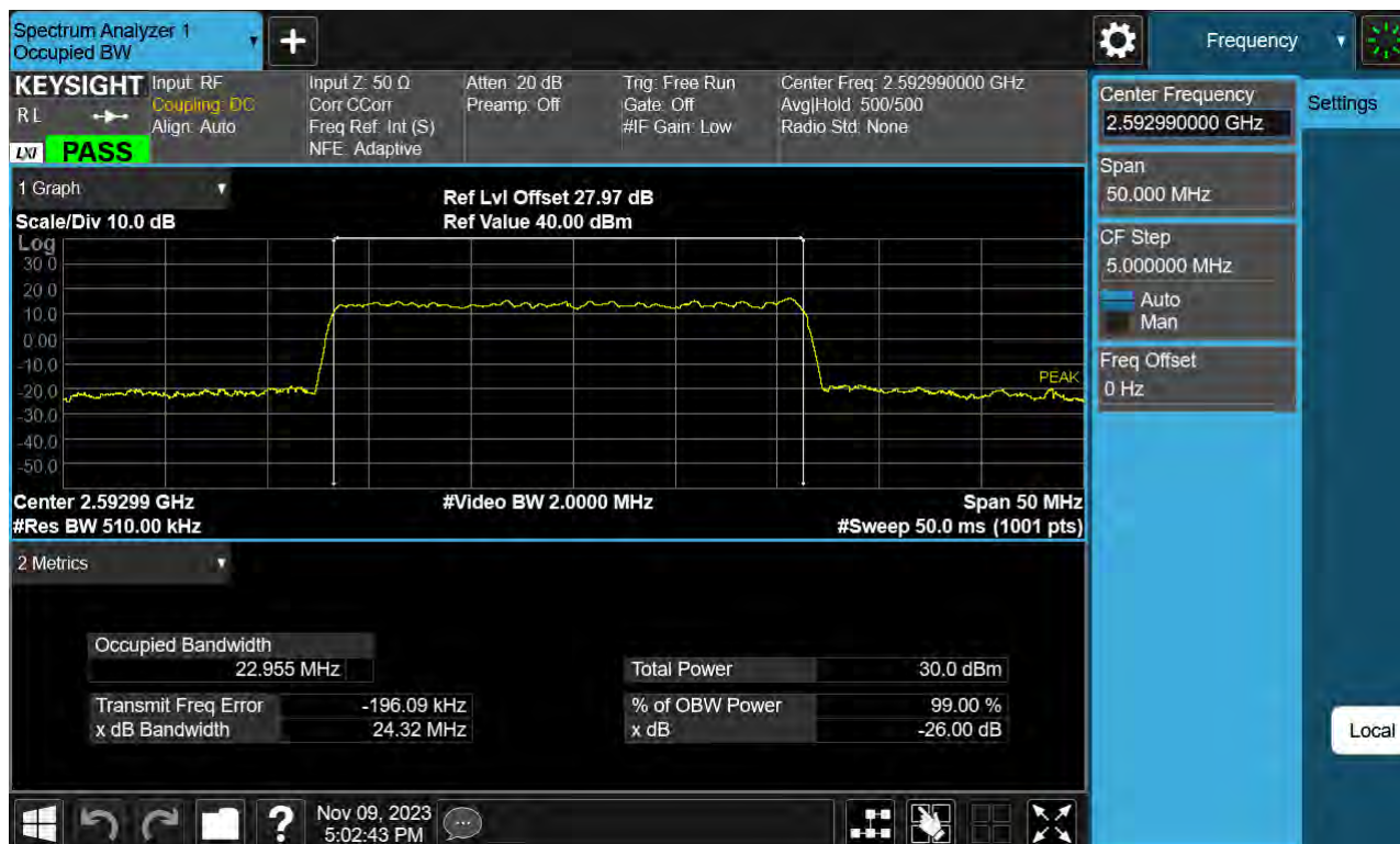
Sub6 n41. Occupied Bandwidth Plot (25 MHz Ch.518598 64-QAM )
