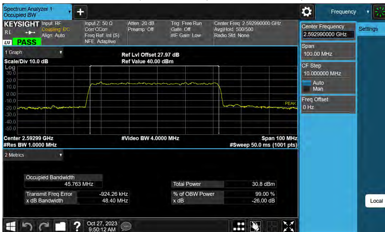
Sub6 n41. Occupied Bandwidth Plot (50 MHz Ch.518598 16-QAM )
