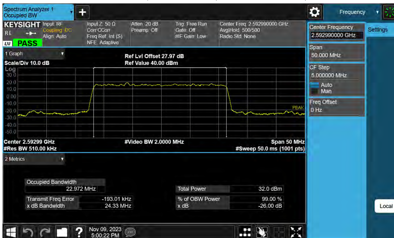
Sub6 n41. Occupied Bandwidth Plot (25 MHz Ch.518598 BPSK )
