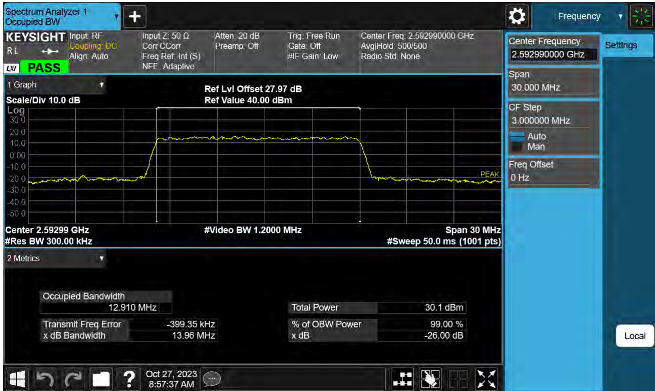
Sub6 n41. Occupied Bandwidth Plot (15 MHz Ch.518598 16-QAM )
