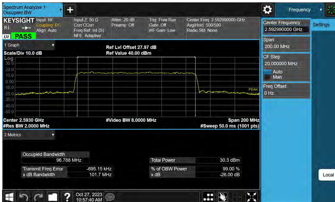
Sub6 n41. Occupied Bandwidth Plot (100 MHz Ch.518598 64-QAM )
