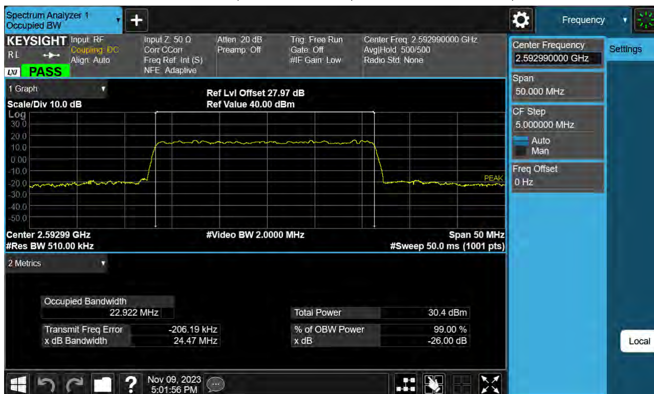
Sub6 n41. Occupied Bandwidth Plot (25 MHz Ch.518598 16-QAM )
