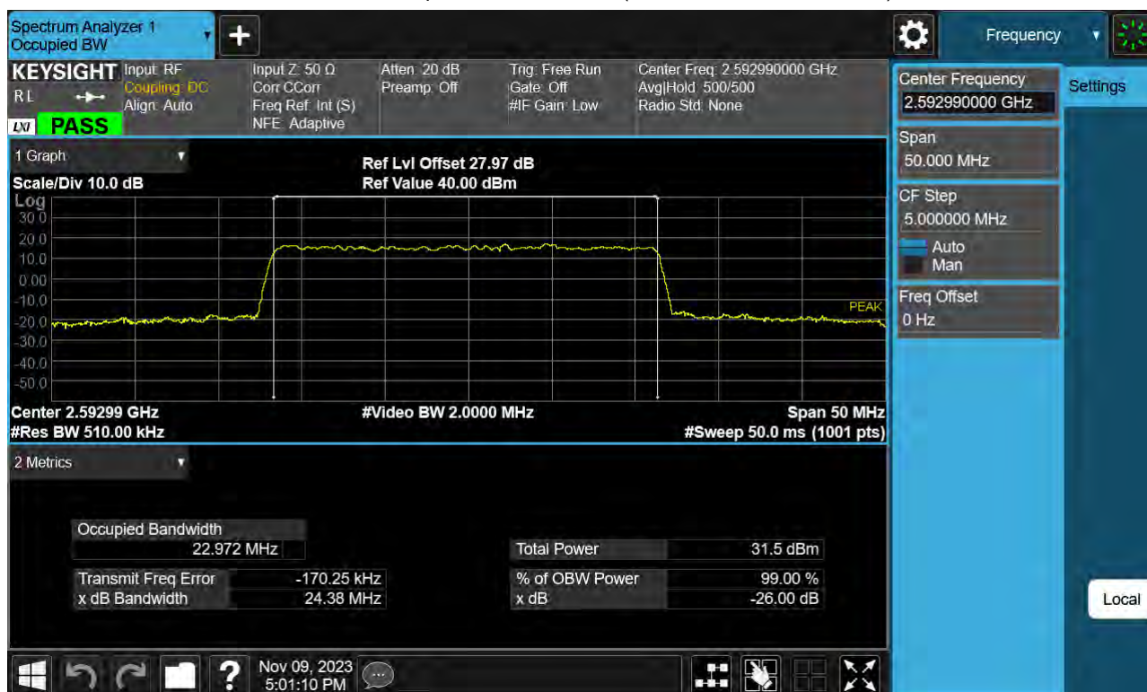
Sub6 n41. Occupied Bandwidth Plot (25 MHz Ch.518598 QPSK )
