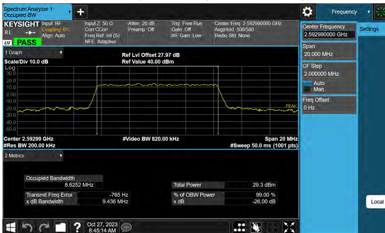
Sub6 n41. Occupied Bandwidth Plot (10 MHz Ch.518598 64-QAM )
