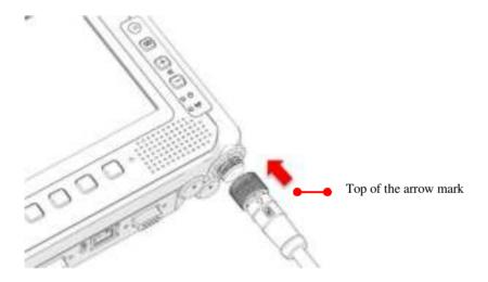
3. Twist the nut to lock the power connector to the device.
