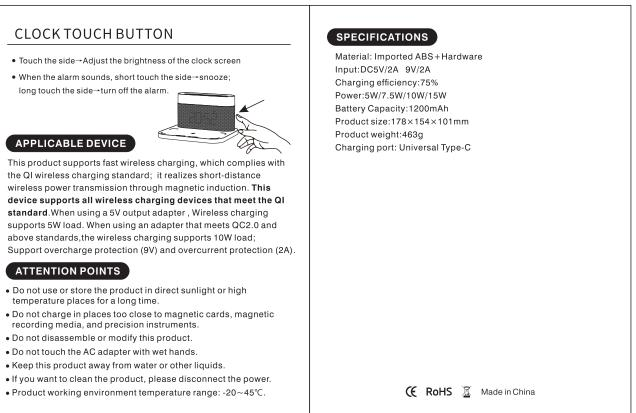
This product supports fast wireless charging, which complies with the QI wireless charging standard; it realizes short-distance wireless power transmission through magnetic induction. This device supports all wireless charging devices that meet the QI standard.When using a 5V output adapter , Wireless charging supports 5W load. When using an adapter that meets QC2.0 and above standards, the wireless charging supports 10W load; Support overcharge protection (9V) and overcurrent protection (2A)
