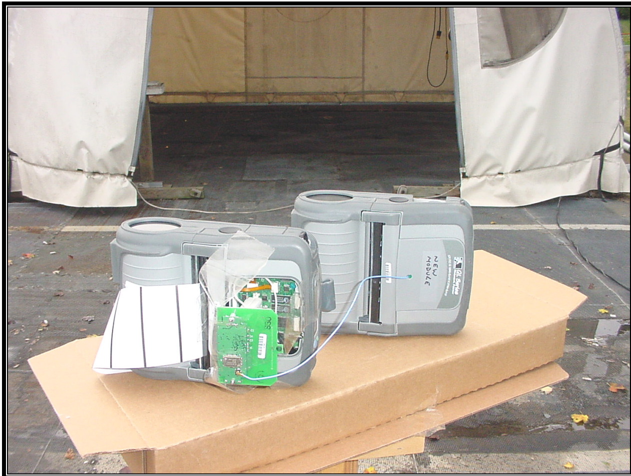
PHOTOGRAPH 16: RADIATED EMISSION FRONT VIEW, WORST CASE CONFIGURATION QL FAMILY SECOND GENERATION BLUETOOTH (CQ17383-1) ANTENNA
