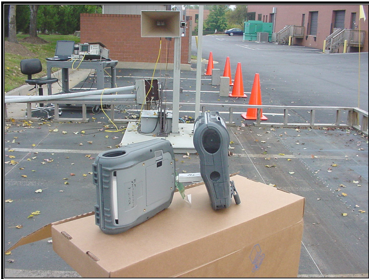
PHOTOGRAPH 13: RADIATED EMISSION REAR VIEW, WORST CASE CONFIGURATION QL FAMILY (CC16203-2) ANTENNA
