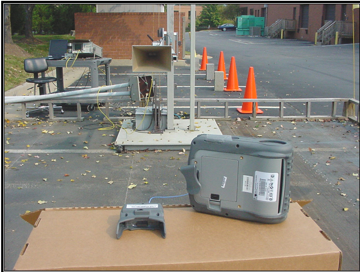
PHOTOGRAPH 15: RADIATED EMISSION REAR VIEW, WORST CASE CONFIGURATION ZPR MODULE (CQ15813-1) ANTENNA
