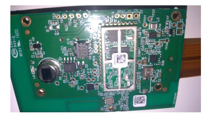
Photograph No.7 916.5 MHz radio board with shield removed
