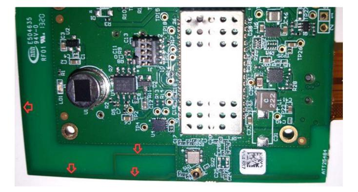
Photograph No.6 ES700MDS-US-M03 the 916.5 MHz radio board front view
