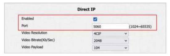
• Port: Set the port for direct IP calls. The default is 5060, with a range from 1-65535. If you enter a value within this range other than 5060, ensure consistency with the corresponding device for data transmission.
