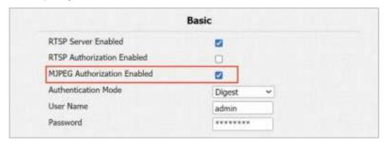
• MJPEG Authorization Enabled: Once enabled, accessing the door phone's real-time image or video by entering the URL into the browser requires verification of the Authentication Mode, User Name, and Password.
