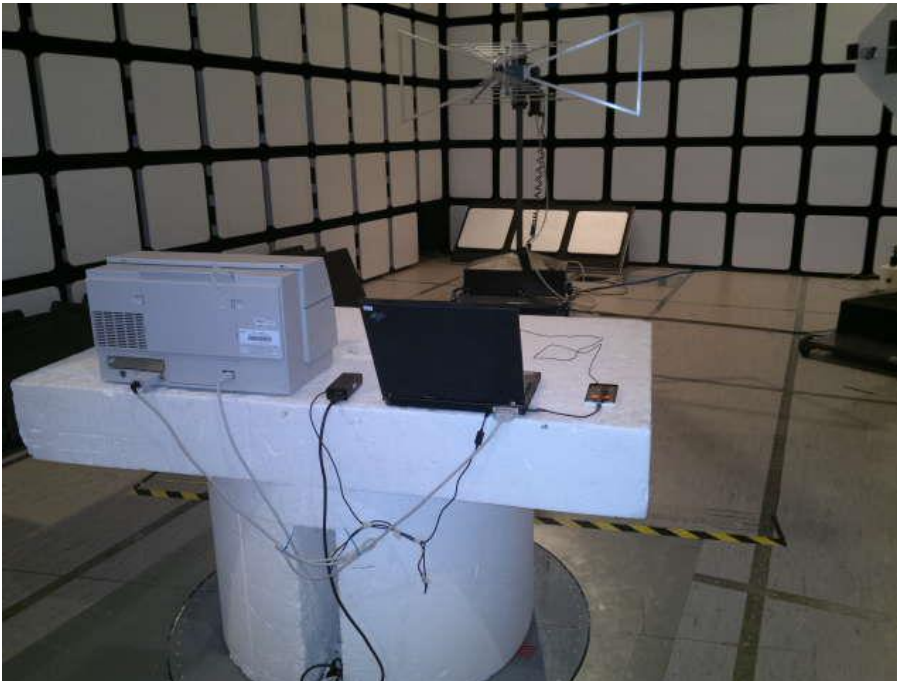
Picture 2. FCC Part 15B Radiated emissions
