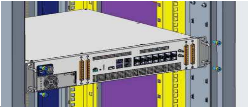
Figure 29. Installation Diagram of DCU in the Rack
