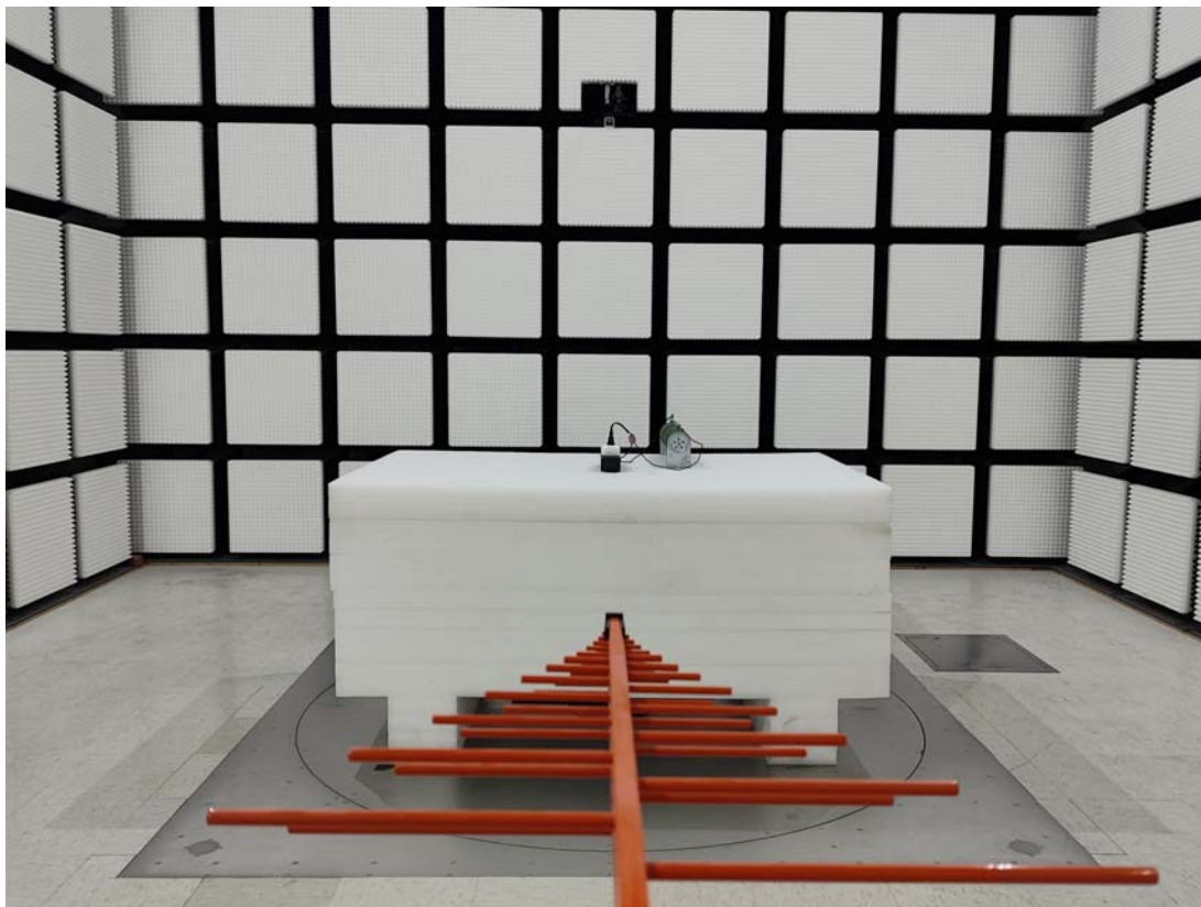
Radiated Emission Above 1GHz View
