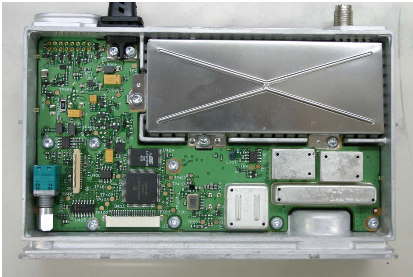
Figure 9-4: Top View of PCB placed in chassis with shield covering transmitter section.
