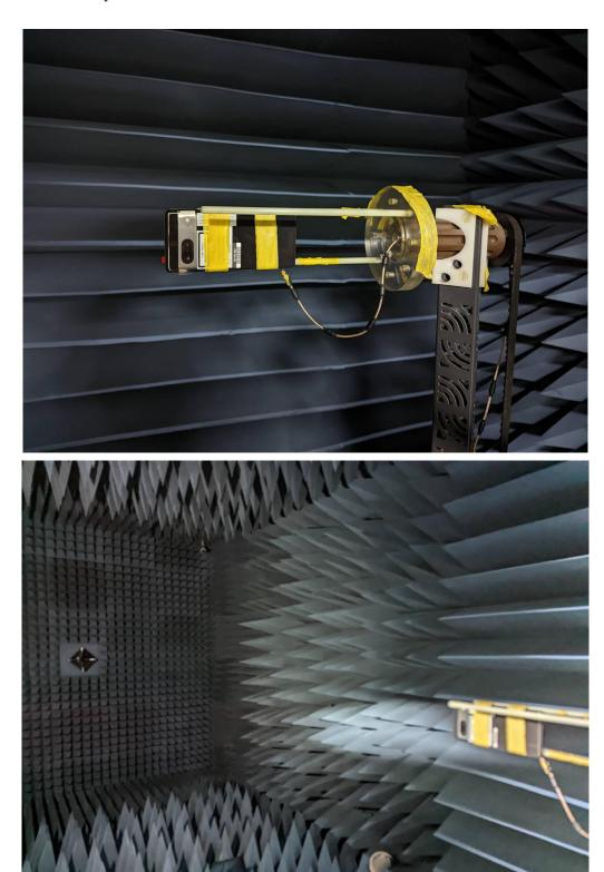
Using the Great Circle Cut Method to obtain the shared gain measurements.
