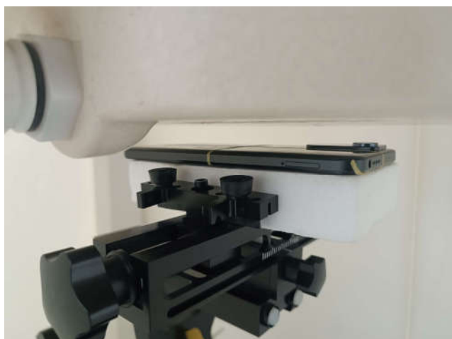
Back, Test Separation 15 mm(sensor off)
