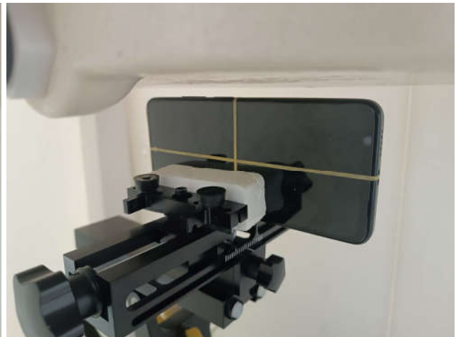
Right Side, Test Separation 10 mm
