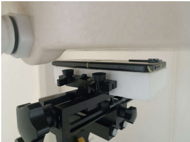
Back, Test Separation 15 mm(sensor off)
