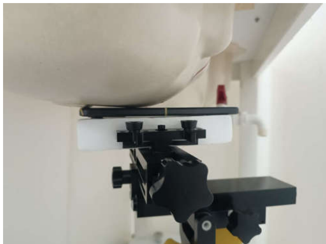
Right Cheek, Test Separation 0 mm
