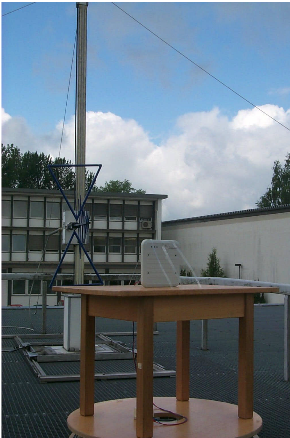
30052ff2.jpg Test set-up final emission measurement (30 MHz to 1 GHz)
