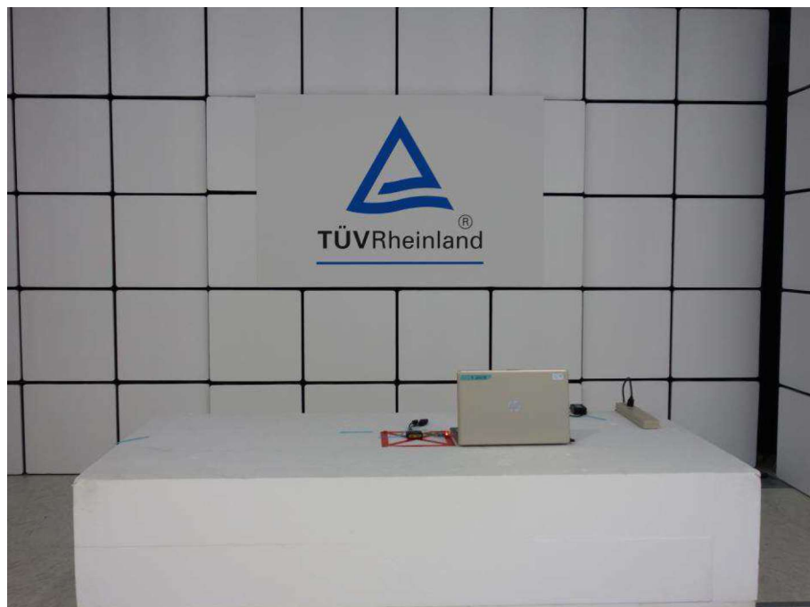
Photograph 2: Set-up for Spurious Emissions (Front View 2)
