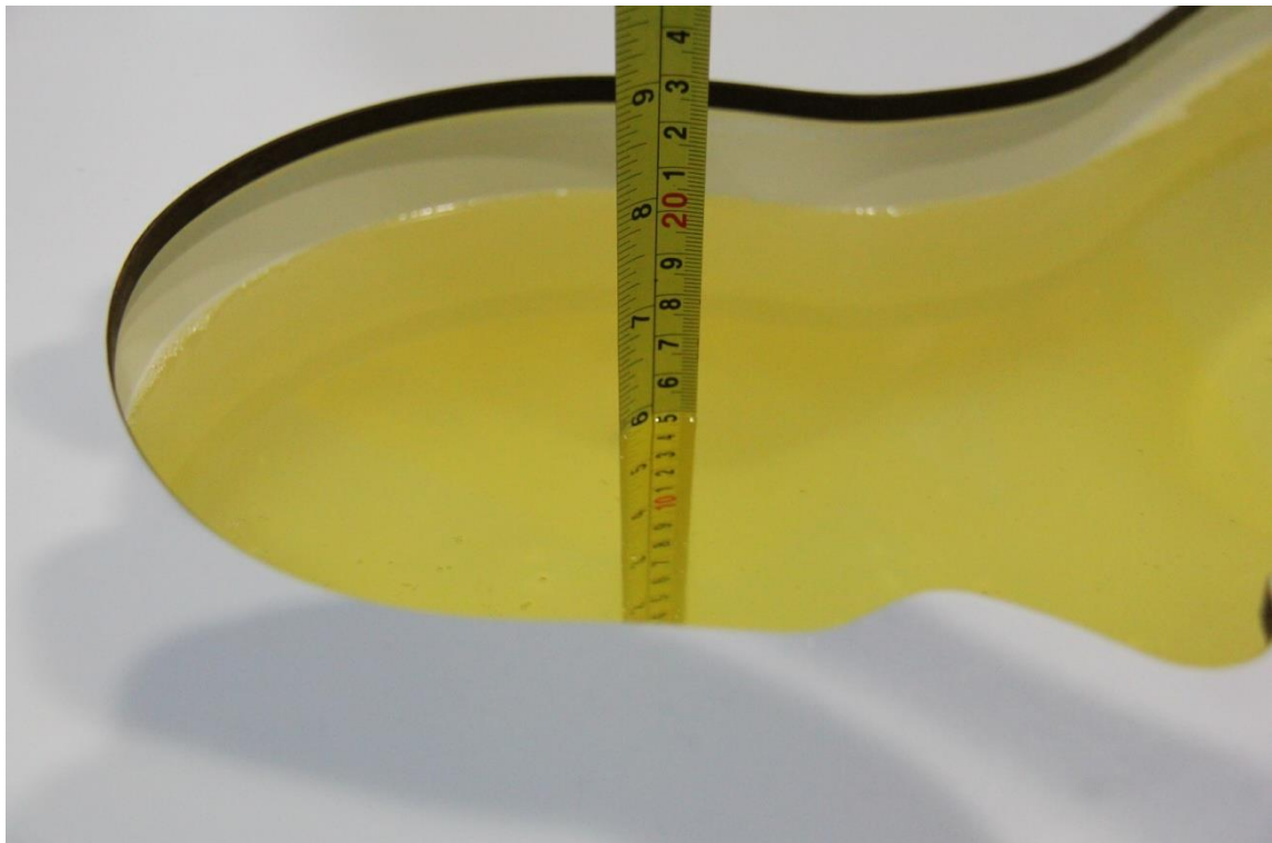
Picture 7-3 Liquid depth in the Head Phantom (2450MHz)
