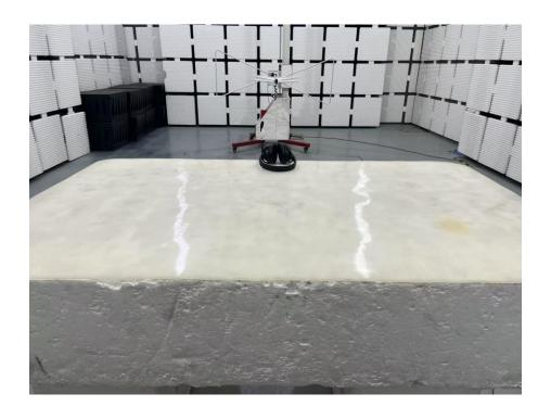
Set-up for Radiated Spurious Emission, Above 1GHz
