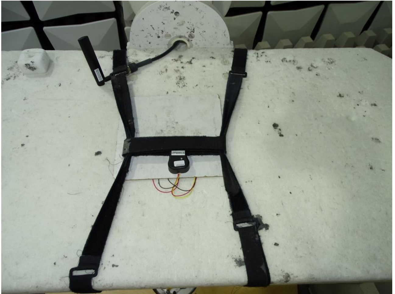
Photo 6: Test setup for radiated measurements, detailed view (1 GHz – 24 GHz; FCC 15c247)
