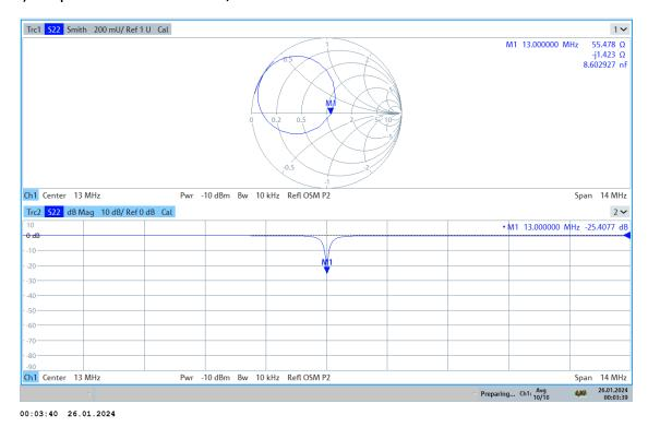
• Return/Loss is greater than the -20 dB cutoff and Impedance is within 5  $\Omega$  of previous value.
