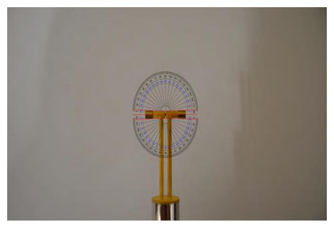
$\bullet~$  The center red line indicates that the arms of the dipole fall within  $\pm 2^{\circ}$
