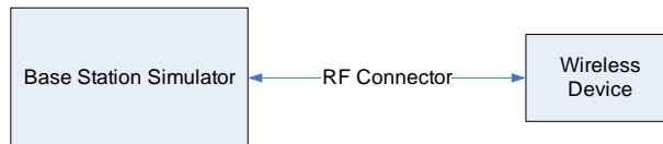
Figure 9-2 Power Measurement Setup
