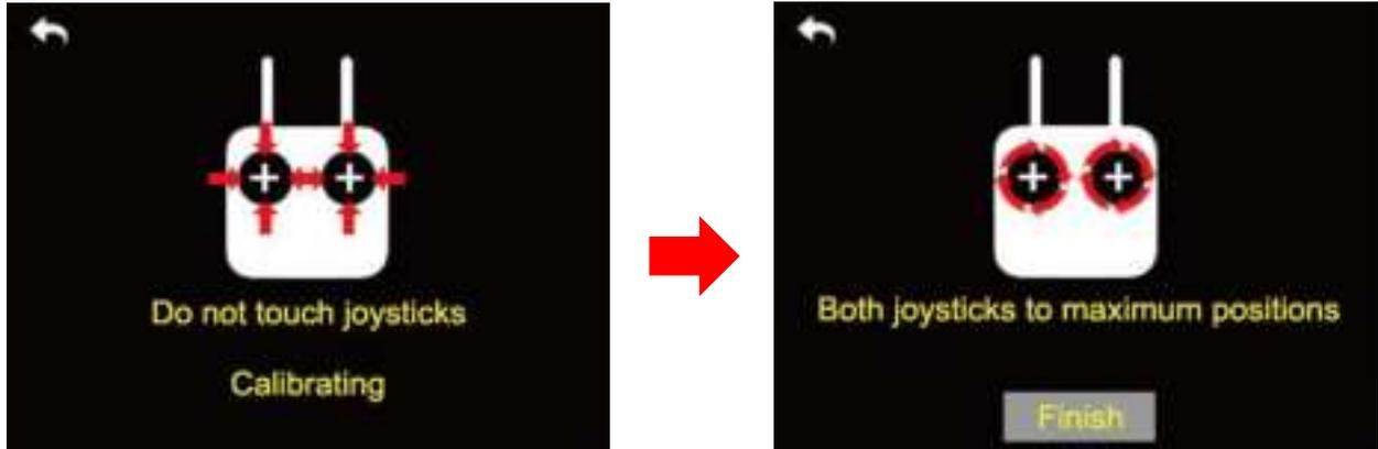
6. When the detecting is finished, push both joysticks to the maximum position and move them in circle for several times;
