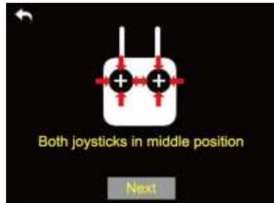
4. Hold the joysticks and make them stay in the middle position (the joystick's tick mark aligns with the transmitter's tick mark), then tap on “Next”;
