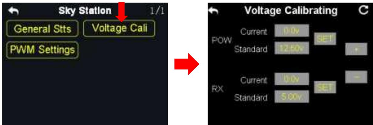
Before using the sky station, it is necessary to calibrate the telemetry voltage of both the sky station and the aircraft.
