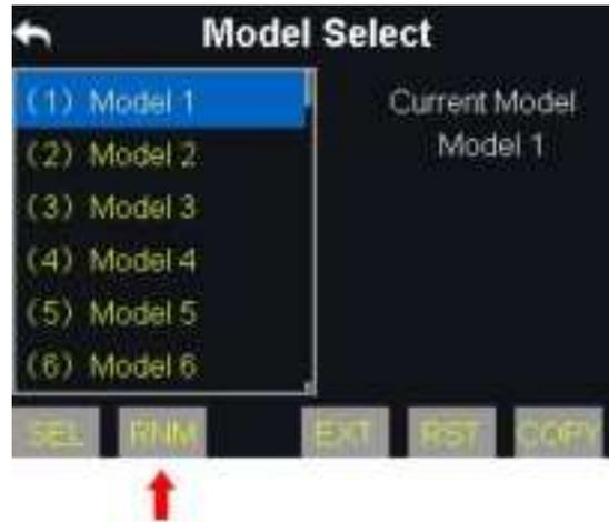
2. Input a new name for the model by using the virtual keyboard, then tap on “yes” to finish.
