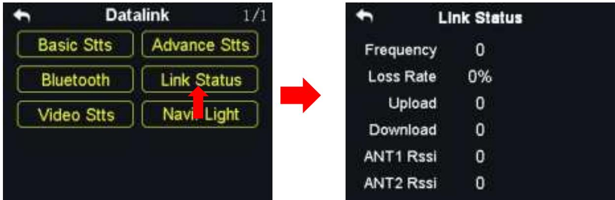
The link status function helps users check the detail signal and link status of VD32 transmitter in real-time.
