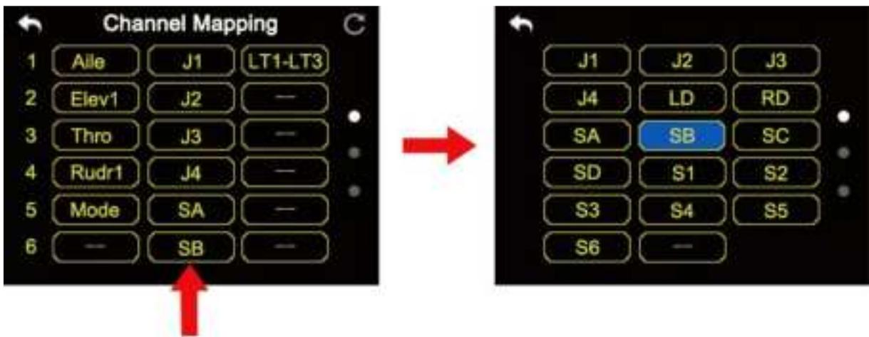
2. In VD32 transmitter system, channel 1-4 is default to be Aileron, Elevator, Throttle, and Rudder.
