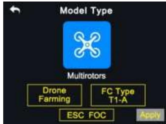
VD32 transmitter supports the function “One Move to Do Agricultural Drone Settings”. Users can select and match the FC (Flight Controller) and ESC (Electronic Speed Controller) type according to what they have bought. Then the joystick/switch/button/dial definition and datalink settings will be done automatically. And you will be ready for flight immediately.
