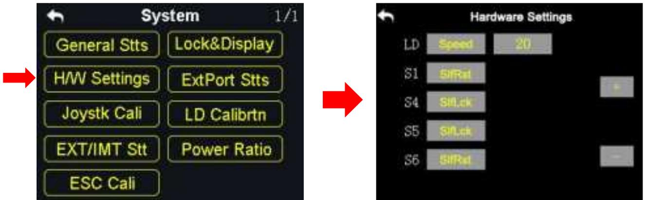
Through the H / W settings users can do advanced settings for the left dial (LD) to switch it between the Position Mode and the Speed Mode and the switch S1 / S4 / S5 / S6 to switch between Self-locking and Self-resetting.
