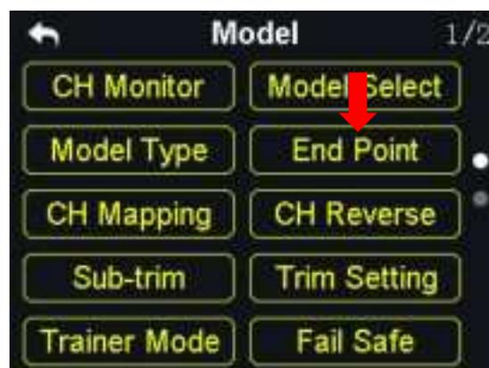
“End Point” function helps users set the output value of a channel and its maximum/minimum limit.
