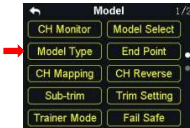
In VD32 transmitter there are several default model types, Fixed-wings / Gliders, Multi-rotors (racing drones, agricultural drones) and the others (helicopters), each model type with its default settings done in advance. Users can choose a model type according to their requirement and customize the settings.
