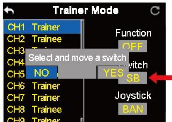
7. When you have defined a switch / button, it will take over the control of turning on / off trainer mode.
