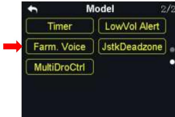
Farming Voice is a professional function is for agricultural drones. The function is supported by up to 6 switches with 16 positions. They are SA, SB, SC, SD, S2 and S3.
