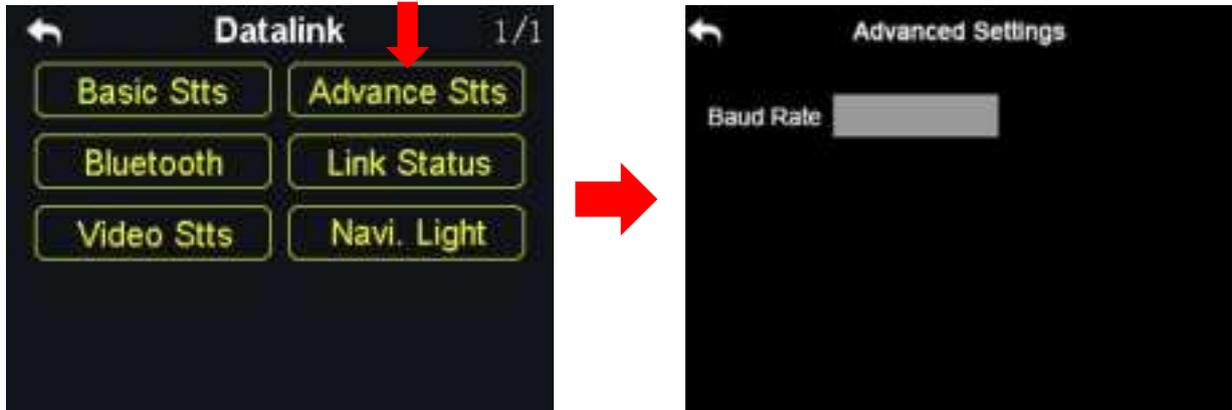
If your flight controller type was not in the list, you can set a baud rate to match your flight controller.
