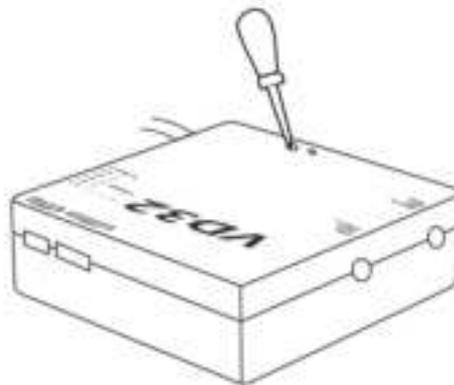
4. Tap on “Link - Start” and wait for a second, if the transmitter indicator and the receiver both blink green, linking is finished.
