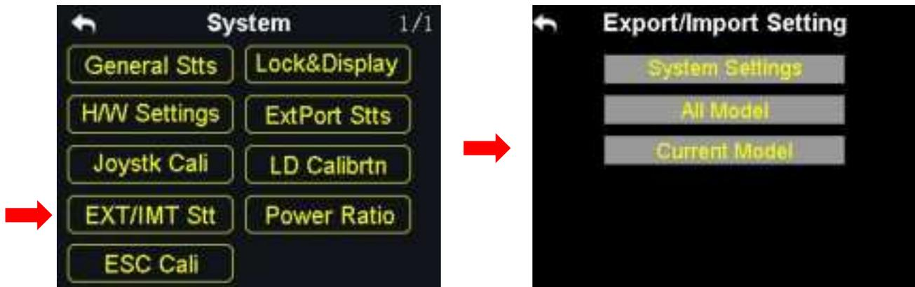
Through the export setting function users can export the data of system settings and model settings to the SD card so as to share the data to another VD32 transmitter.
