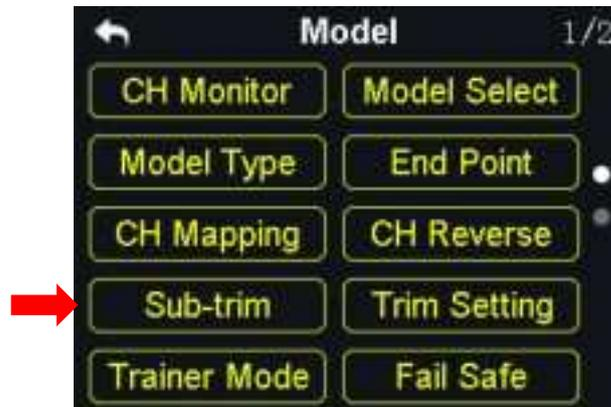
Sub-Trim function helps users set the middle position value of a channel's and do trim adjustment to the aircraft's flight attitude.
