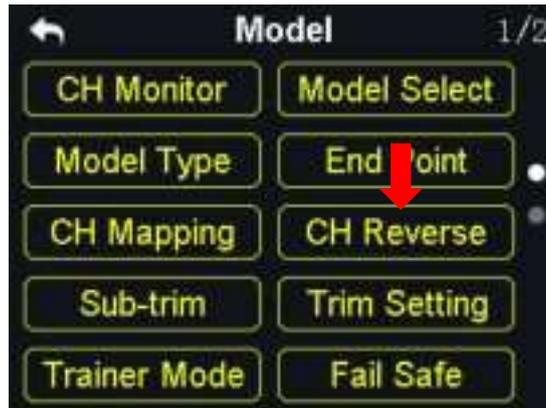
Users can reverse a channel’s output direction through “Channel Reverse”.
