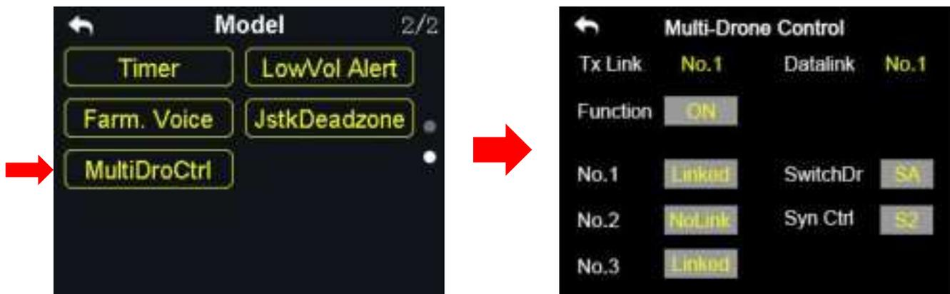
Through one VD32 transmitter users can control up to three drones at the same time.
