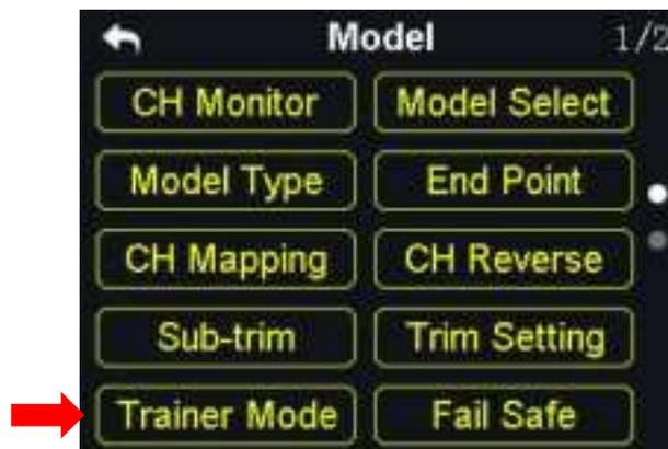
VD32 transmitter’s trainer mode helps experienced users train new talents. In the trainer mode, two transmitters are connected by a trainer cable. The users can decide which channel to use for training.
