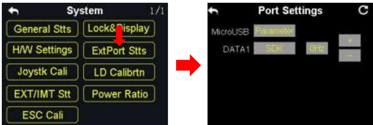
The extending ports function help users extend transmitter function to external hardware devices and SDK. Currently VD32 transmitter supports a Micro-USB port, a USB port and a 4-Pin Groove Port (DATA1).
