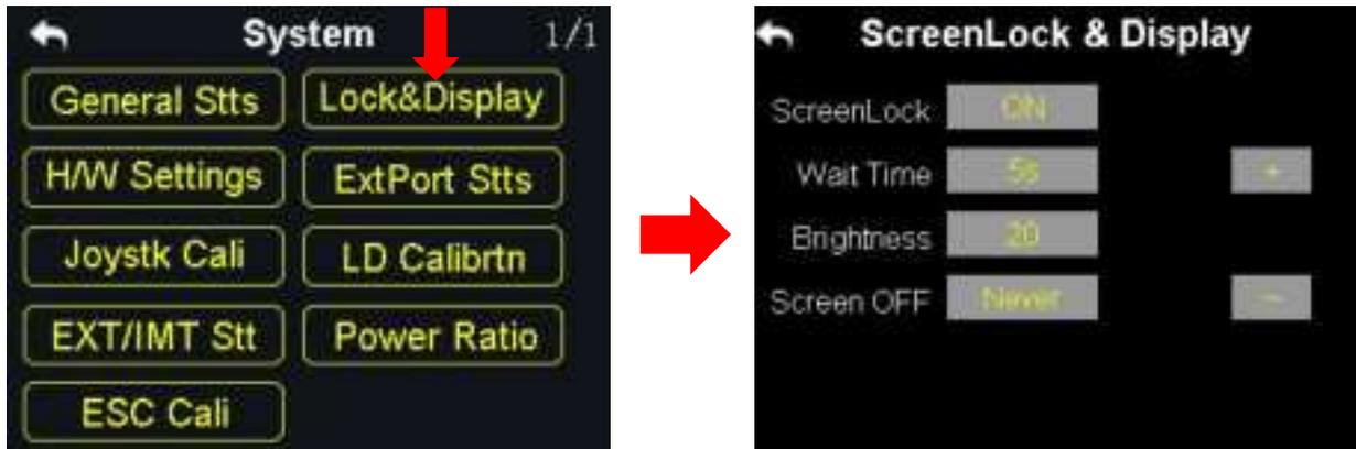
Users can turn on / off the screen lock, set the waiting time, adjust the screen brightness and the screen sleep waiting time of VD32 transmitter.
