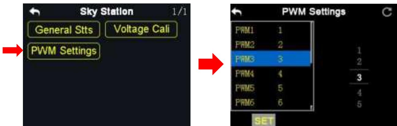
In VD32 transmitter and the PWM mode, users can redefine the output channel of the sky station (channel 1-9 in default), so that if the channel 9 is already working in SBUS or PPM mode, the PWM ports 1 to 8 can still output to the channels 1 to
