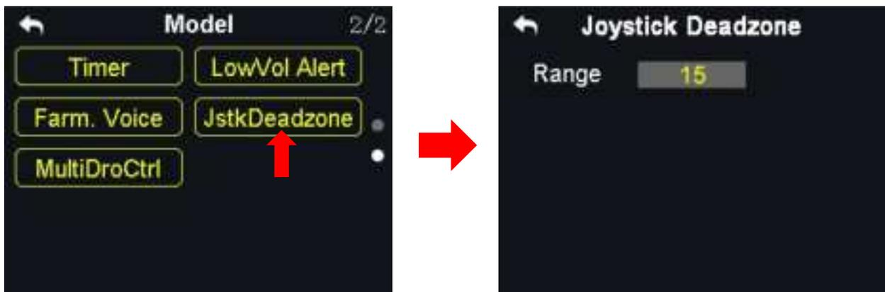
By setting a certain dead zone range, VD32 transmitter helps user filter out channel values which are input by touching the joysticks unintentionally.
