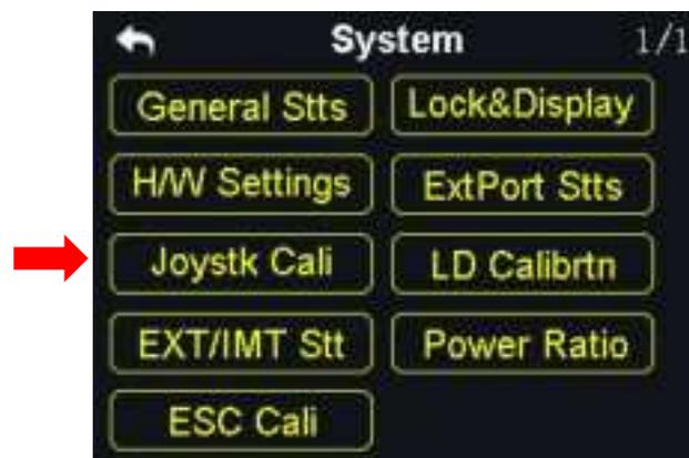
The Joystick calibrating function help users calibrate the joysticks' middle position. Regular calibration can maintain the control accuracy of the joysticks.
