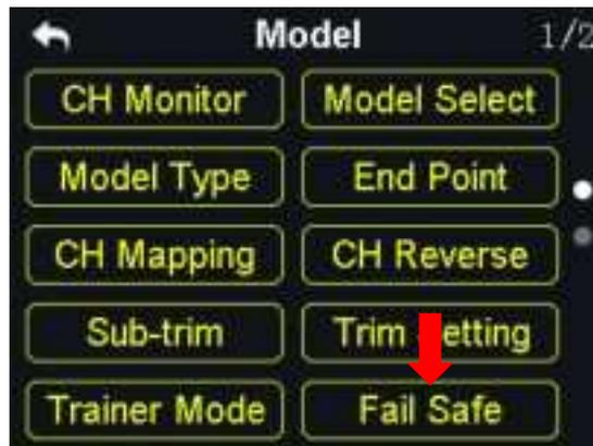
Before linking VD32 transmitter to VD32 receiver, do not forget to do fail-safe settings and turn on the function, thus if your transmitter lost linkage with receiver, fail-safe function will run automatically and immediately to protect your model from a crash.
