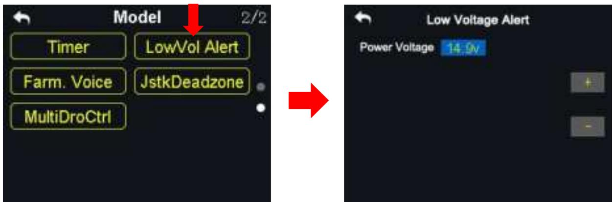
When the user's aircraft power voltage is lower than the safe level, VD32 transmitter will vibrate and send voice alert.
