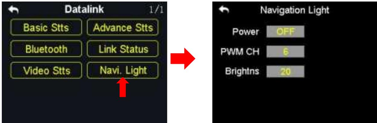
Users can power on/off the navigation light on the drone.
