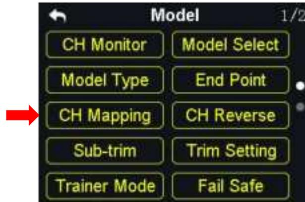
All 16 channels of VD32 transmitter can be mapped freely as you need to the joysticks, switches, buttons, and dials.
