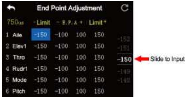
2. When the channel output is normal, tap on the left/right box to input value of the minimum/maximum limit, the range is between -150 and 150.
