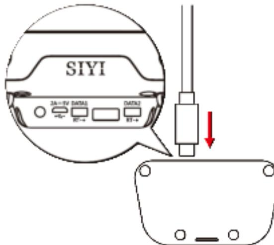
Please use the original OTG Micro-USB cable coming in VD30 packing list for connecting the Micro-USB port on bottom transmitter to the USB port on the charger adapter. When the charging indicator is solid red, transmitter is under charging. When the charging indicator turns to solid green, charging is finished.
