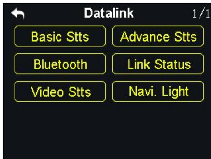
**Basic Stts (Basic Settings):** Set basic functions of the datalink module.
