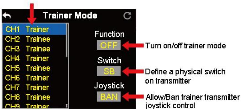
4. The transmitter with the trainer mode turned on is the master transmitter, the other one is the slave transmitter; in the master transmitter the channel is default to be “Trainer”;
