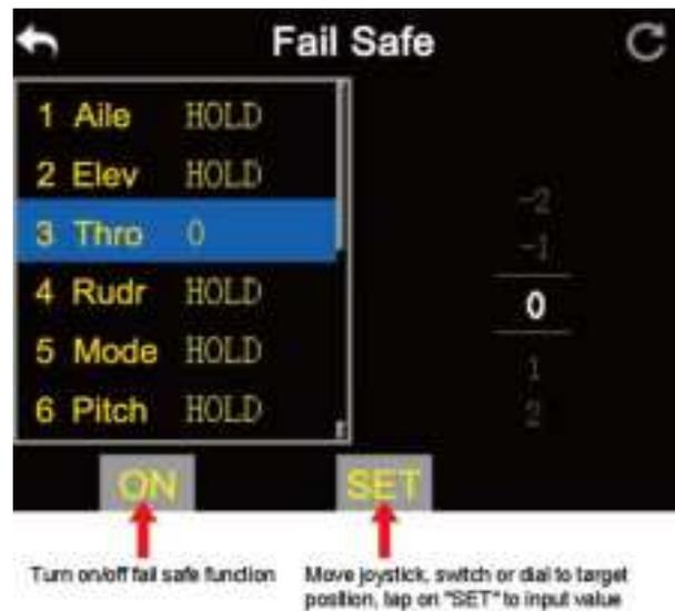
4. Tap on “OFF” and switch it to “ON” to activate Fail-Safe function.
