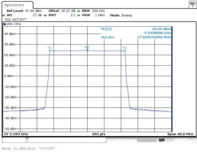
Figure 24 Occupied Bandwidth – 64QAM (2593.0 MHz) (20MHz Channel BW)
