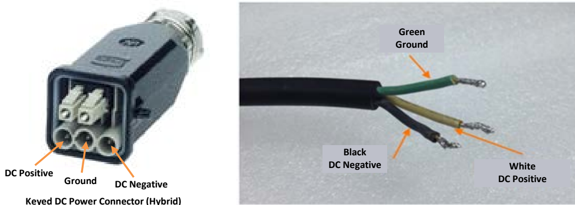
Figure 8: Hybrid Connector Direct DC Power Connection Polarity
