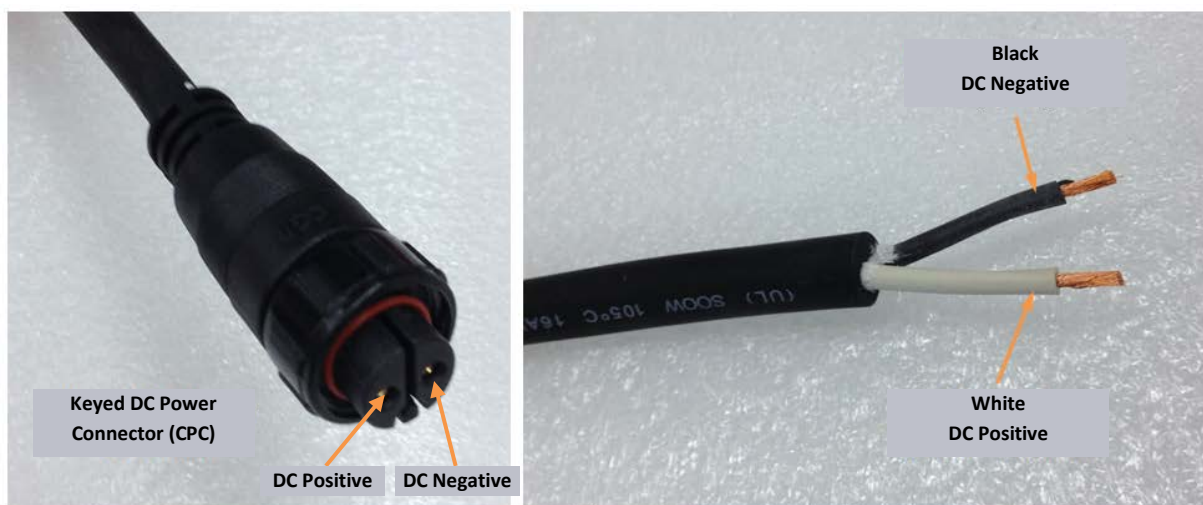
Figure 7: Direct DC Power CPC Connector Connection Polarity
