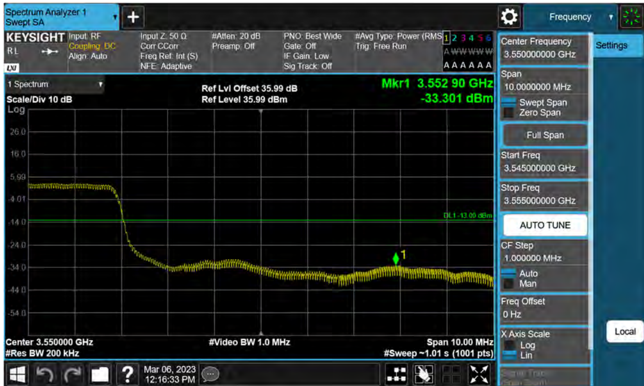
Sub6 n77(78). High Band Edge Plot (40 M BW Ch.635332 BPSK FullRB)(1)
