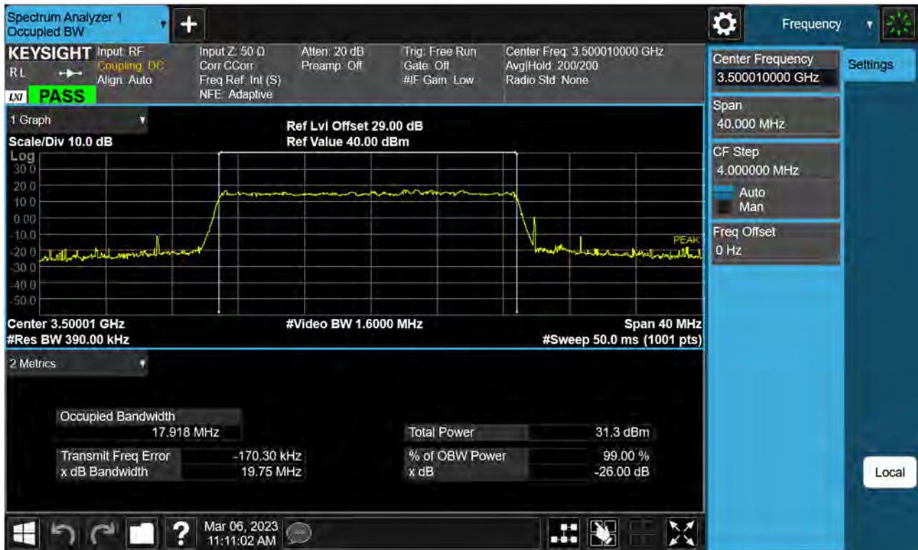
Sub6 n77(78). Occupied Bandwidth Plot (20 M BW Ch.633334 64QAM)
