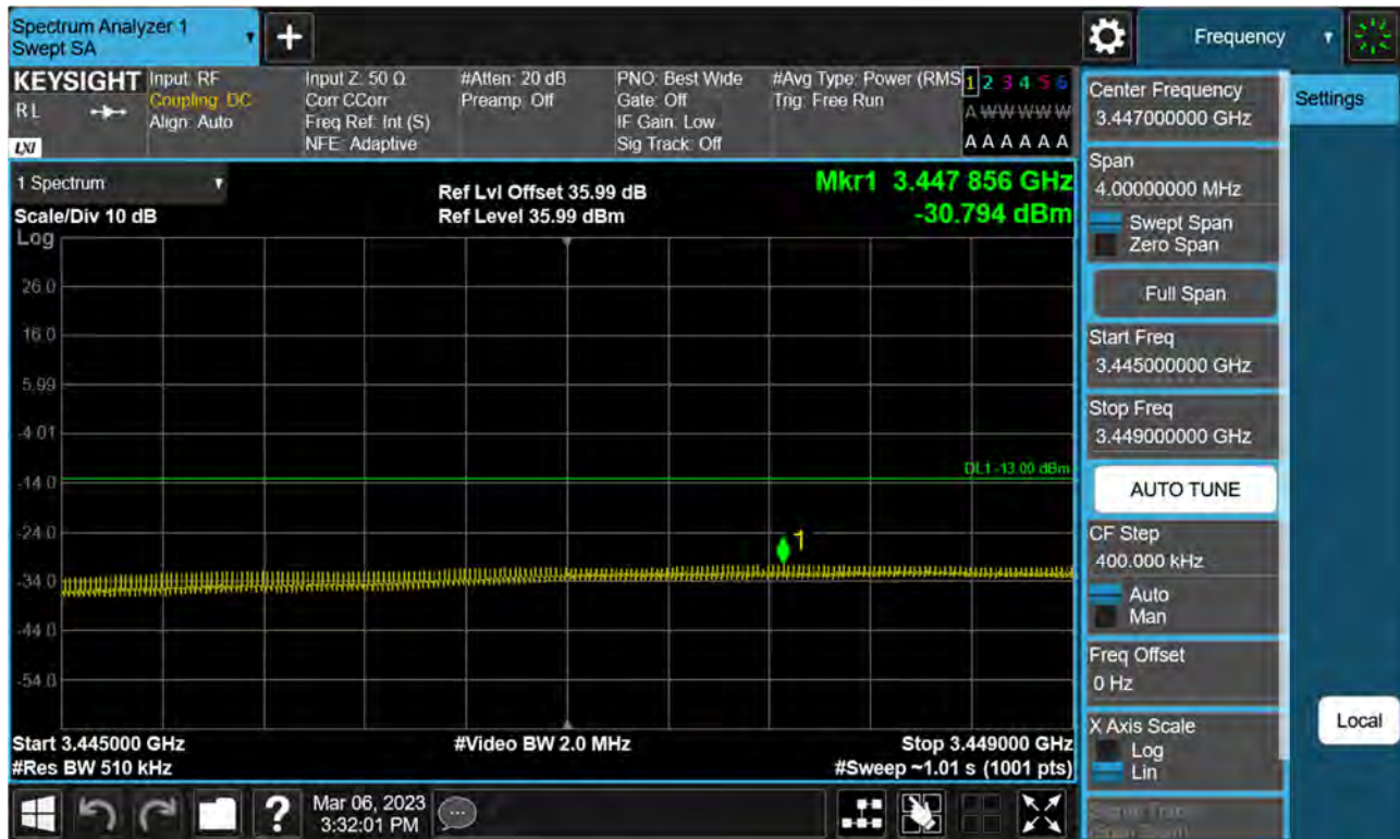
Sub6 n77(78). Low Band Edge Plot (30 M BW Ch.631000 BPSK FullRB)(2)
