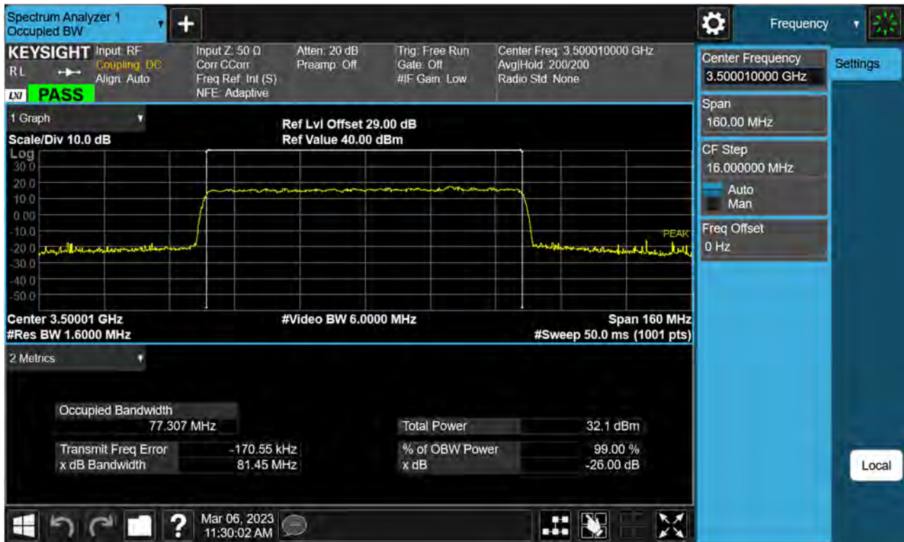
Sub6 n77(78). Occupied Bandwidth Plot (80 M BW Ch.633334 64QAM)
