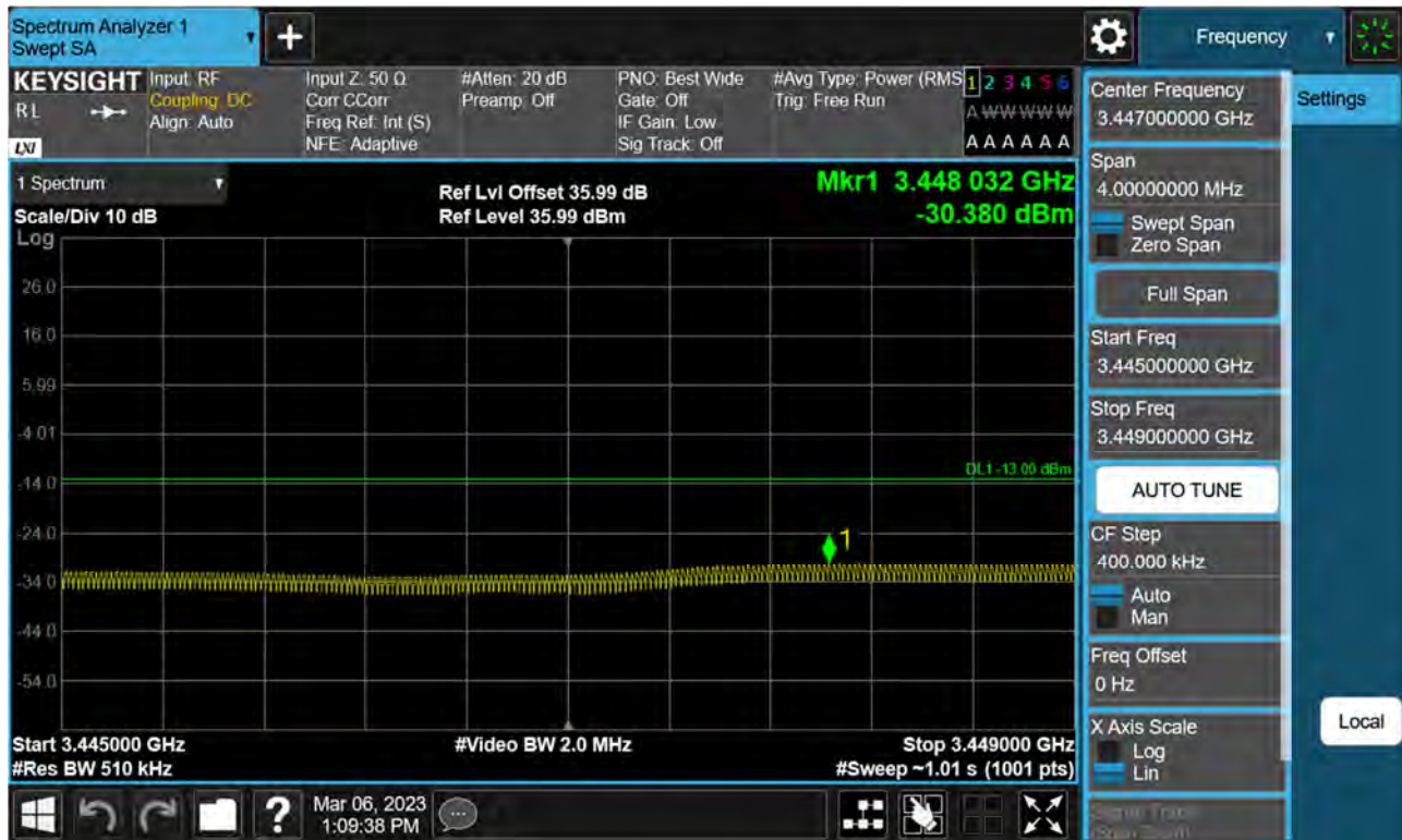
Sub6 n77(78). Low Band Edge Plot (50 M BW Ch.631668 BPSK FullRB)(2)
