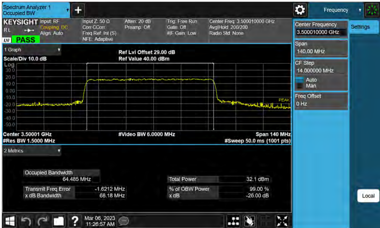
Sub6 n77(78). Occupied Bandwidth Plot (70 M BW Ch.633334 64QAM )
