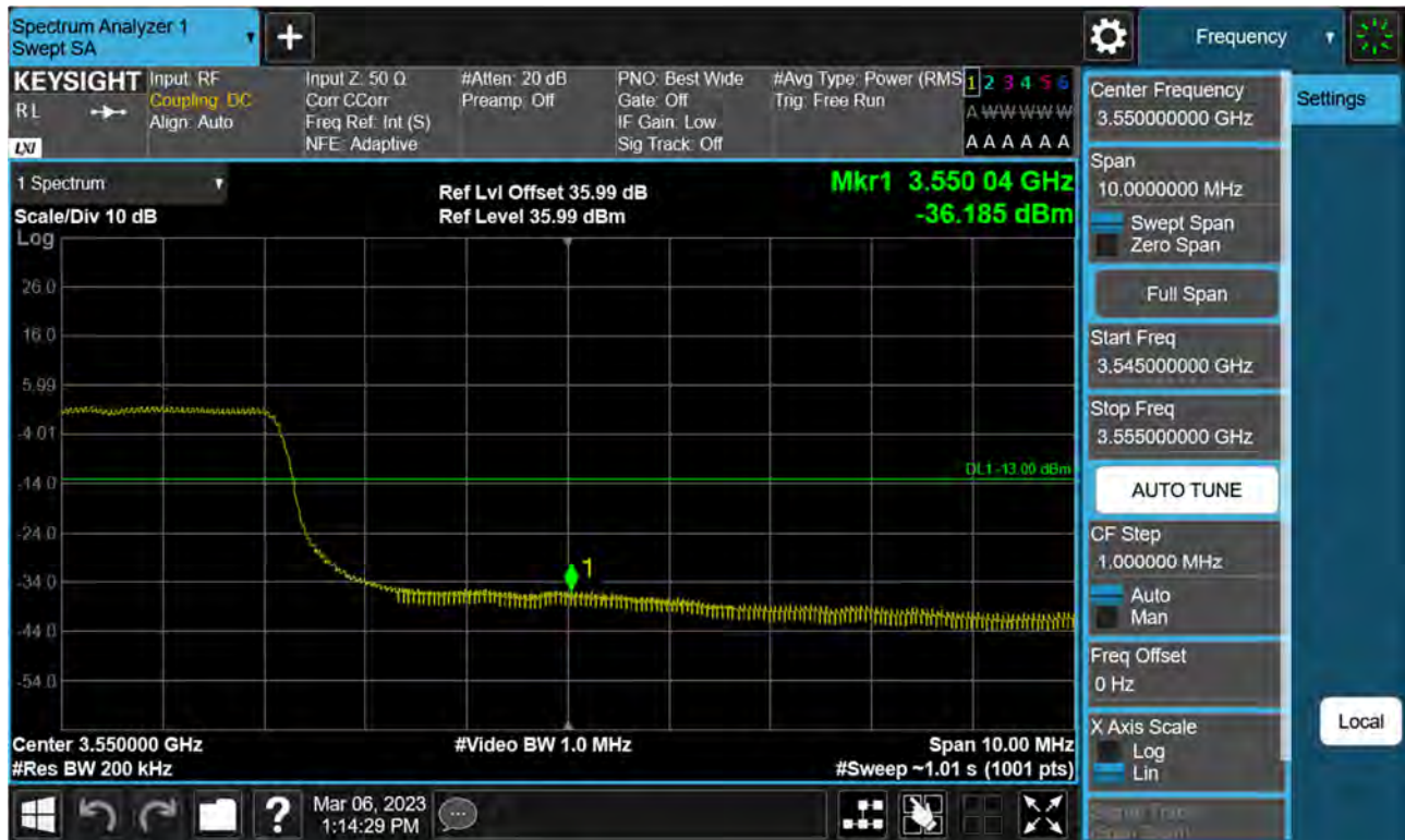
Sub6 n77(78). High Band Edge Plot (50 M BW Ch.635000 BPSK FullRB)(1)
