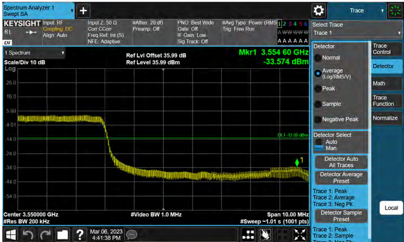
Sub6 n77(78). High Band Edge Plot (30 M BW Ch.635666 BPSK FullRB)(1)
