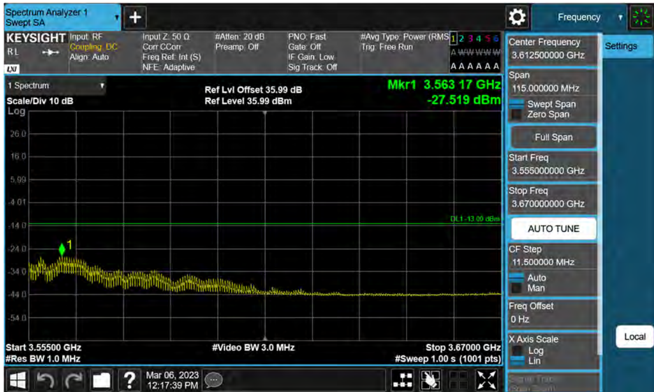
Sub6 n77(78). High Band Edge Plot (40 M BW Ch.635332 BPSK FullRB)(3)
