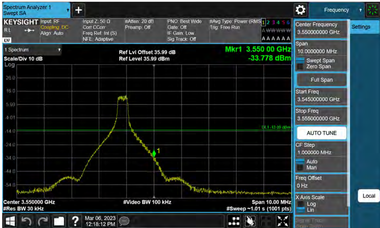
Sub6 n77(78). High Band Edge Plot (40 M BW Ch.635332 BPSK 1RB)(1)
