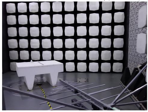
1.4 Radiated Spurious Emissions Test Setup (Above 1GHz)
