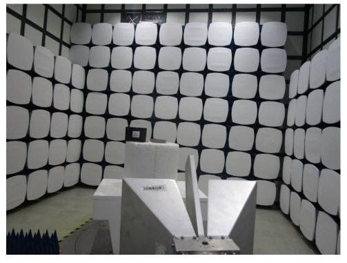
1.3 Radiated Spurious Emissions Test Setup (30MHz-1GHz)
