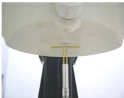
Fig 8.1 Photo of Dipole Setup
