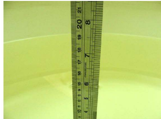
Fig 7.2 Photo of Liquid Height for Body SAR
