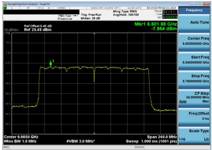
Plot 7-703. LPI Power Spectral Density Plot SDM Primary Antenna WF5B (160MHz 802.11ax RU996x2 (UNII Band 7) - Ch. 143)
