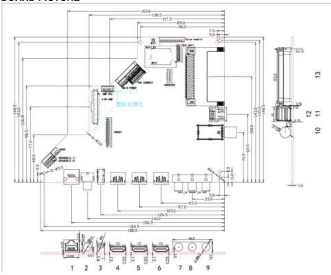
**Size:**  $188 \text{mm}(L)^* 148.5 \text{mm}(W)^* 1.6 \text{mm}(H)$
