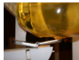
Figure A.4 Left Head SAR Test Setup -- Ear / 15° Tilt Position --
