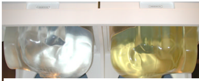
Figure 7.1 Left and Right SAM Phantom shells
