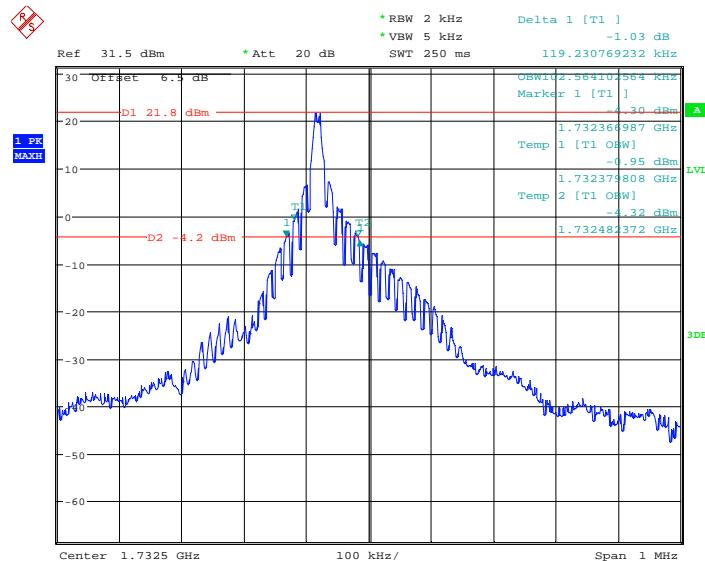
**BPSK (3.75kHz,1#0) - 99% Occupied & 26 dB Emissions Bandwidth, High channel**
