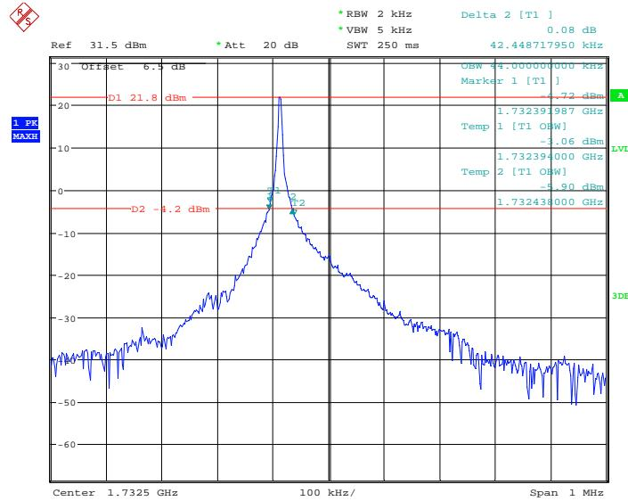
**BPSK (15kHz,1#0) - 99% Occupied & 26 dB Emissions Bandwidth, Middle channel**
