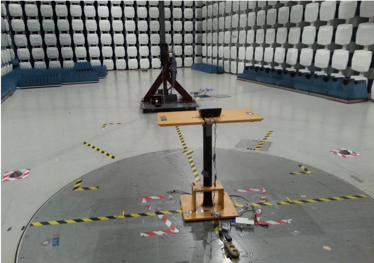
Bluetooth Radiated Emissions Test, \leq 1 GHz
