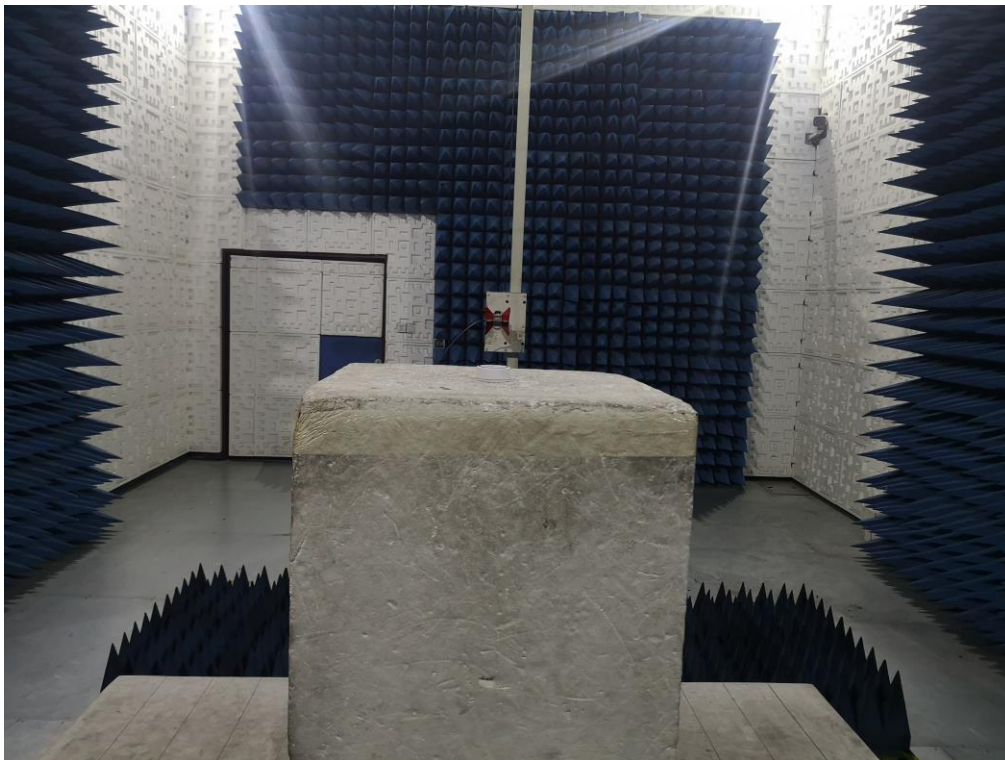
RADIATED EMISSION TEST SETUP ABOVE 1GHZ
