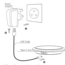
Connect the power adapter to socket.
