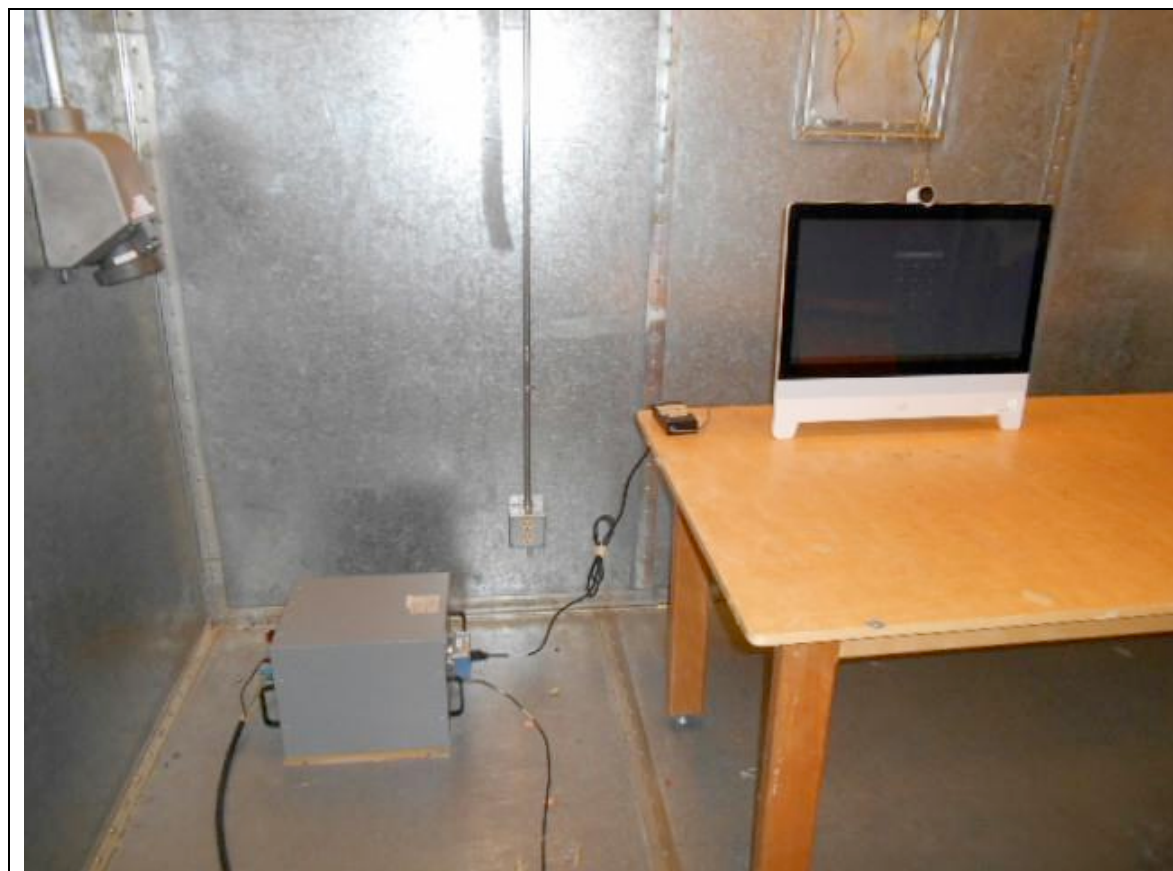
Title: Conducted Emissions Test Configuration
