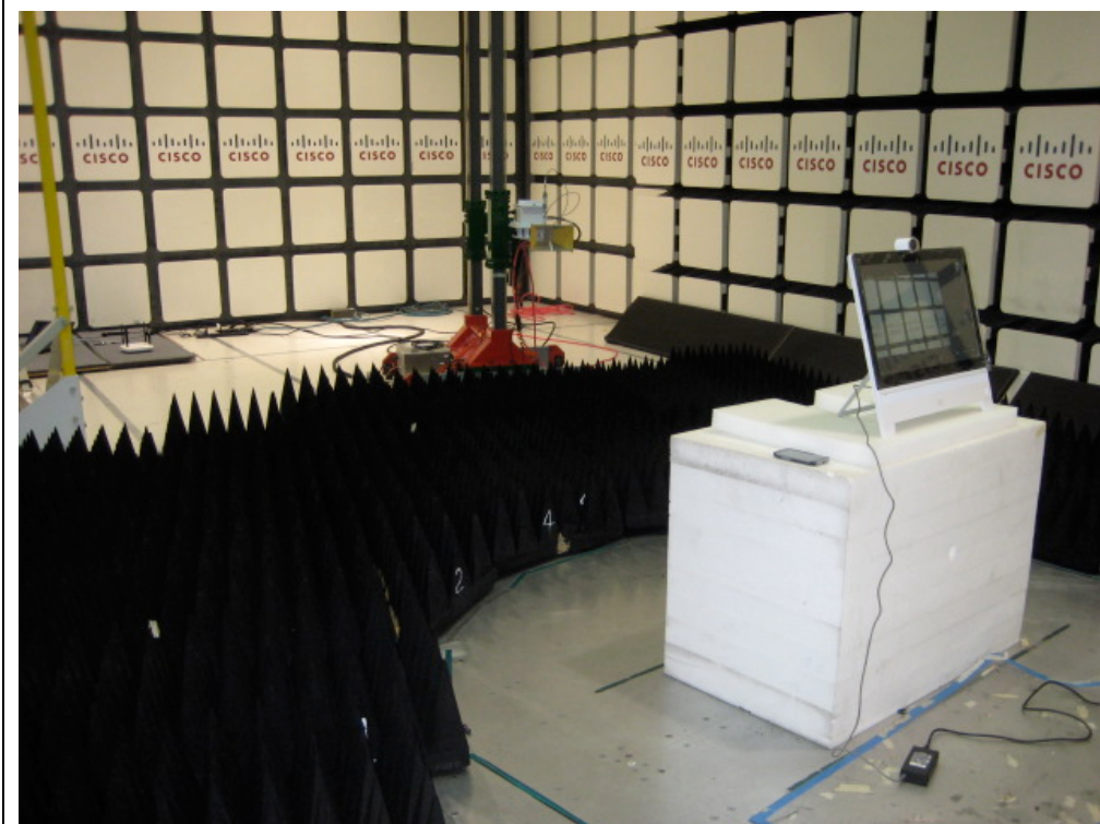
Title: Co-Location Radiated Spurious Emissions 1-18GHz Test Setup
