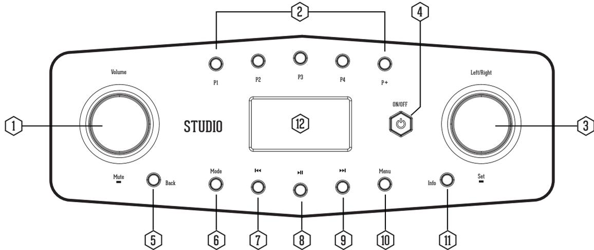
1 **Volume +** :Clockwise is volume up; **Volume -** :Counterclockwise is volume down; **Mute**: A short press will mute the volume. A short press will unmute the volume.
